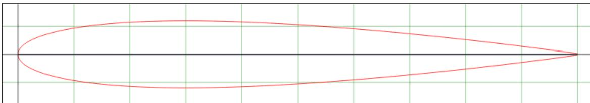
Figura 3. 3 NACA 0012 Airfoil [Airfoil Tools]
