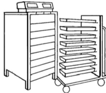
Infrared (regethermic) oven system, 4.7 to 5.0 kW
