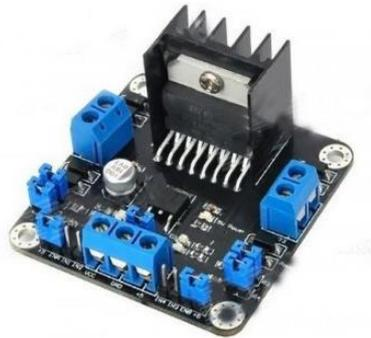
Figura 13.-Módulo Driver Motor de Pasos –Puentes H L298N (Store, 2014)
