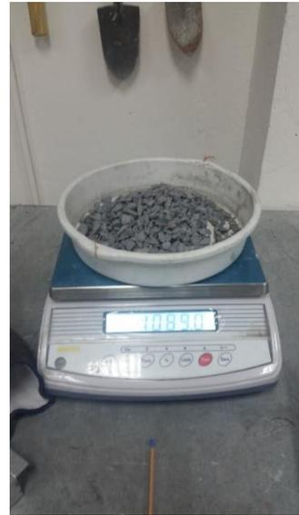
Figura 2.5 PESO SECO SEGÚN ASTM C127-12
