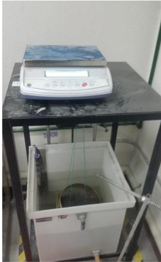
Figura 2.4 PESO SUMERGIDO SEGÚN ASTM C127-12
