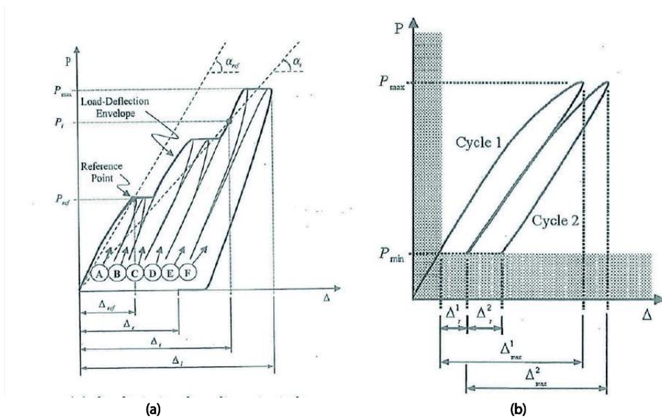
Figure 1. ACI Cyclic loading protocol stop criteria: (a) Deviation from linearity index; (b) Permanency ratio. (ACI Committee 437, 2013)
