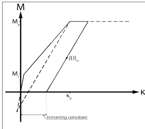
Figure 11. Stiffness from retrograde branch (Vos, 2015)
