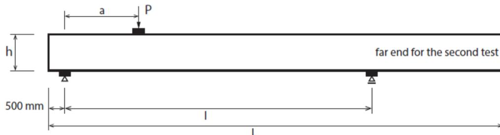
Figure 4. Beam experiments layout
