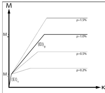
Figure 3. Moment curvature diagram, semi linear approach. (Vos, 2015)
