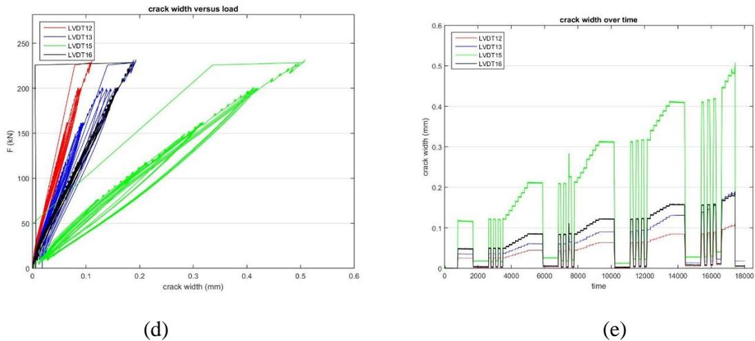
Figure 7. P804A2 experiment results: (a) load-displacement; (b) load-strain; (c) time-strain (d) load-crack width; (e) time-crack width
