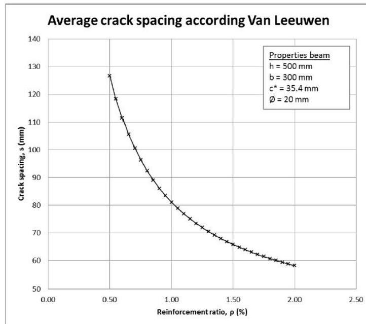
Figure 12: Average crack spacing according to Van Leeuwen (1962)
