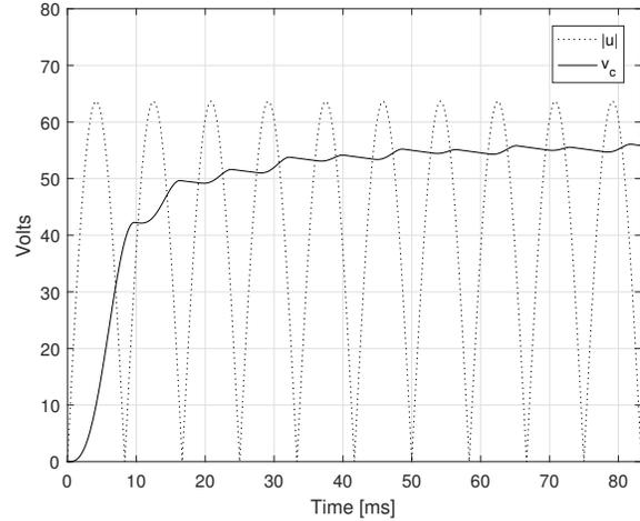
Fig. 2: Rectified mains voltage and capacitor voltage.  $L = 6.6mH$ ,  $C = 3mF$ ,  $R_1 = 1\Omega$ ,  $R_2 = 110\Omega$ ,  $V_s = 45V$
