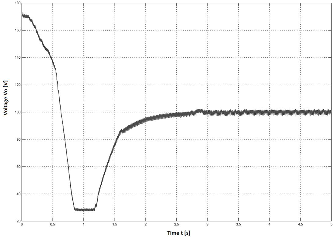
Fig. 19: Simulation result for the three-phase rectifier control system. Set point of 100 [V]
