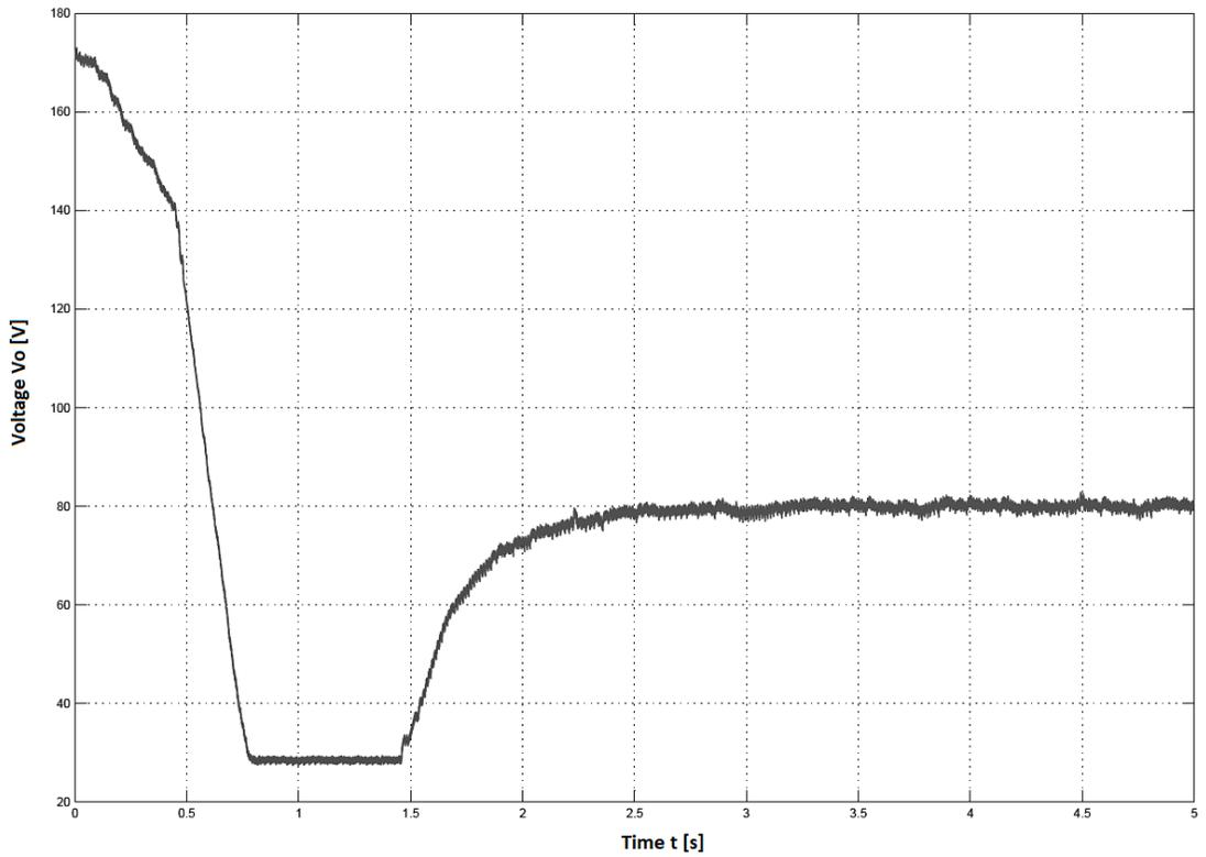
Fig. 20: Simulation result for the three-phase rectifier control system. Set point of 80 [V]
