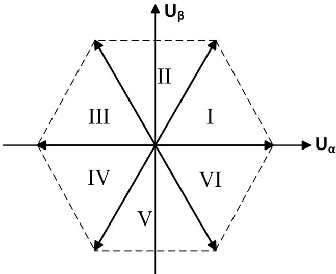
Fig. 12: Hexagon sectors in space vector modulation
