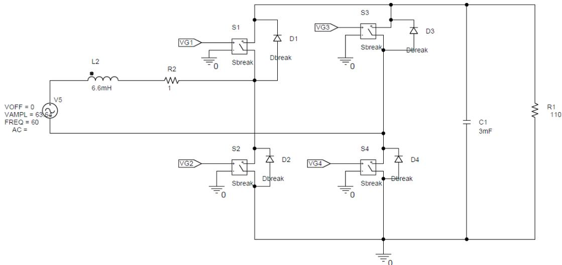
Fig. 14: Controlled single-phase rectifier
