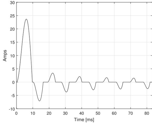
Fig. 3: Inductor current.  $L = 6.6mH$ ,  $C = 3mF$ ,  $R_1 = 1\Omega$ ,  $R_2 = 110\Omega$ ,  $V_s = 45V$
