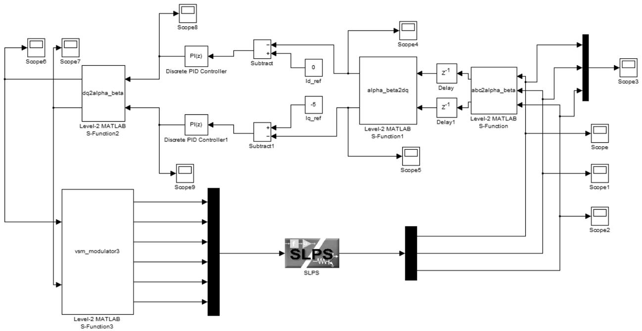
Fig. 22: Simulink model of the current control loop for the inverter.
