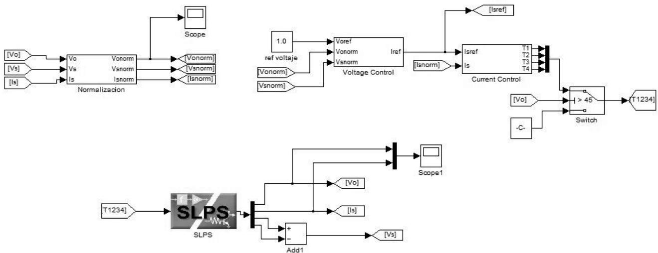
Fig. 15: Single-phase rectifier voltage control diagram in Simulink
