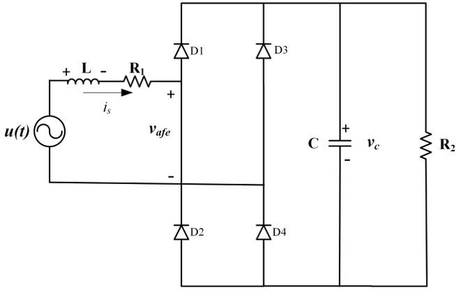
Fig. 1: Single-phase line commuted rectifier
