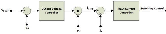
Fig. 8: Control scheme of the single-phase rectifier
