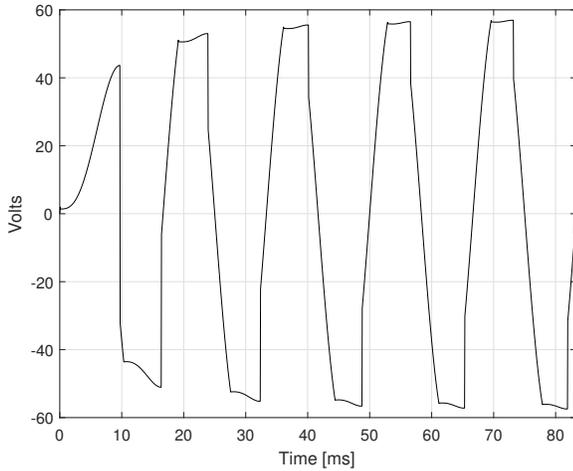
Fig. 4: Rectifier input voltage.  $L = 6.6mH$ ,  $C = 3mF$ ,  $R_1 = 1\Omega$ ,  $R_2 = 110\Omega$ ,  $V_s = 45V$
