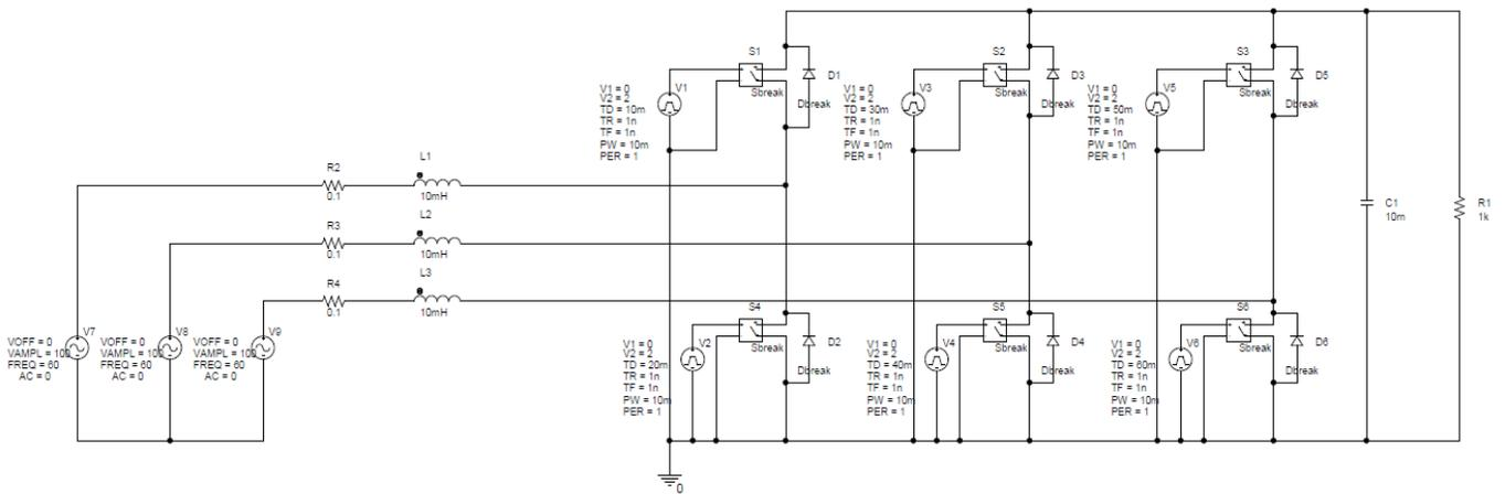
Fig. 18: Three-phase rectifier circuit in PSpice
