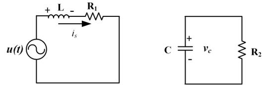
Fig. 6: Equivalent circuit for diodes and switches active simultaneously
