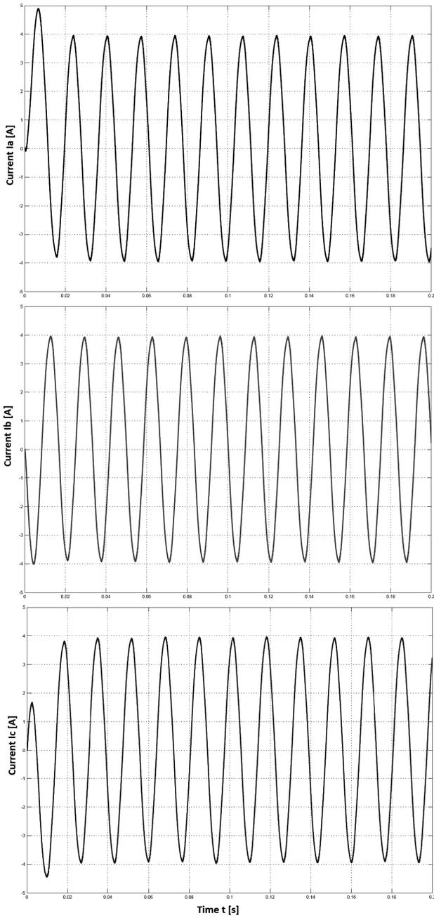
Fig. 23: Simulation result for the three-phase inverter control system. Set point of 4[A]
