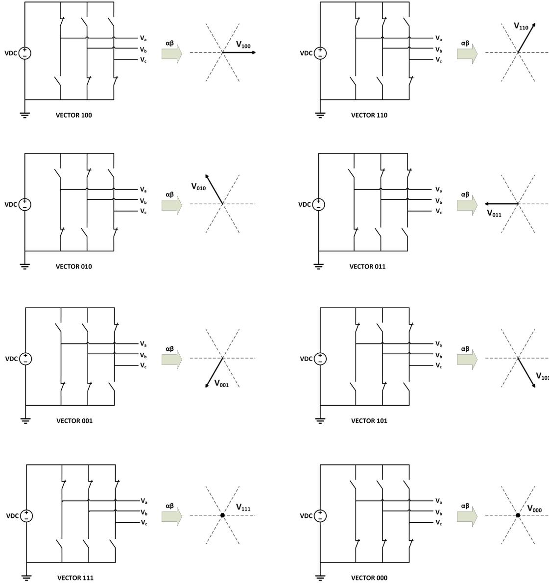
Fig. 11: Possible output voltage vectors for the three-phase inverter
