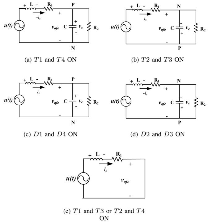
Fig. 7: Equivalent circuits for regenerative rectifier ( $v_c(t) \leq |u(t)|$ ).
