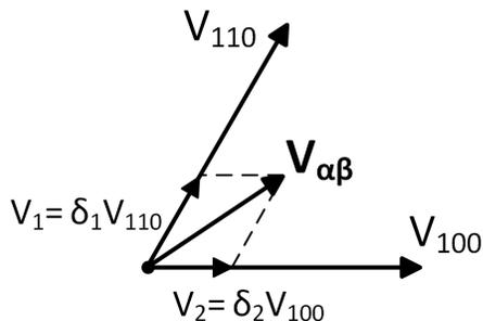
Fig. 13: Projection of the desired voltage in the fundamental vectors
