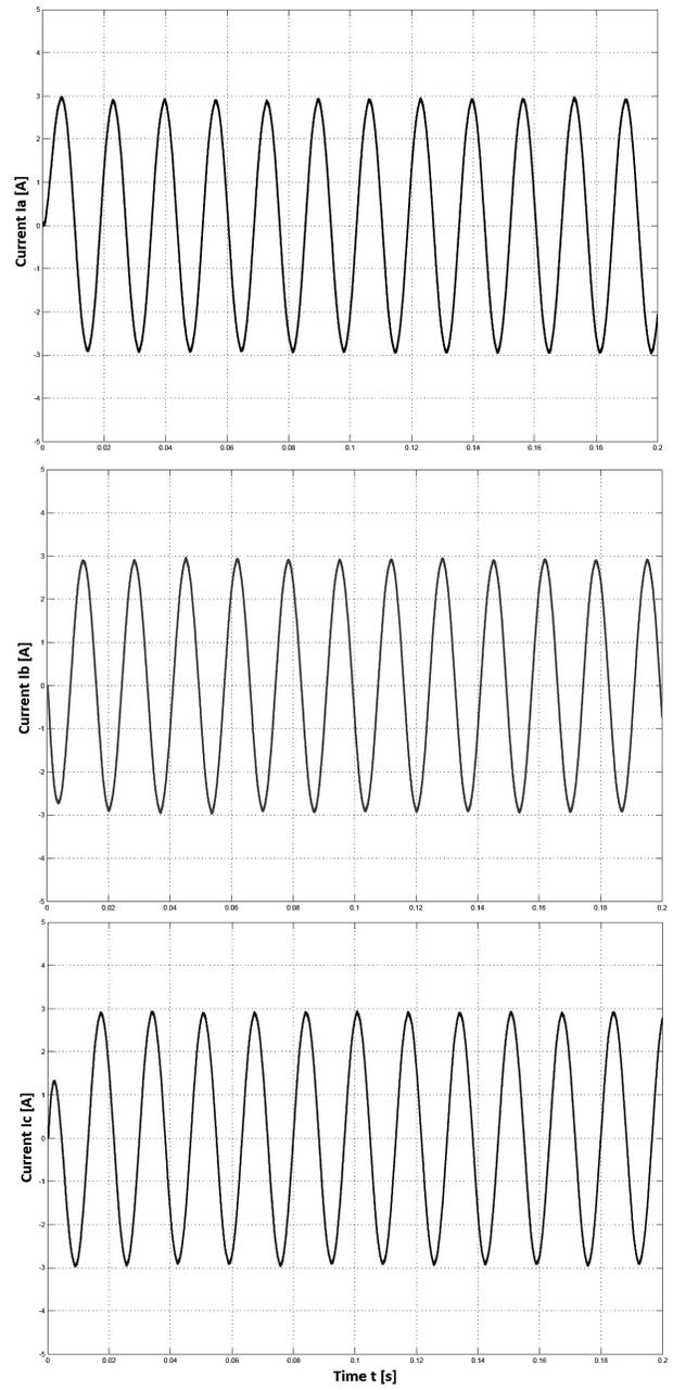
Fig. 24: Simulation result for the three-phase inverter control system. Set point of 3[A]
