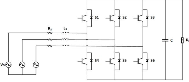
Fig. 9: Three-phase rectifier
