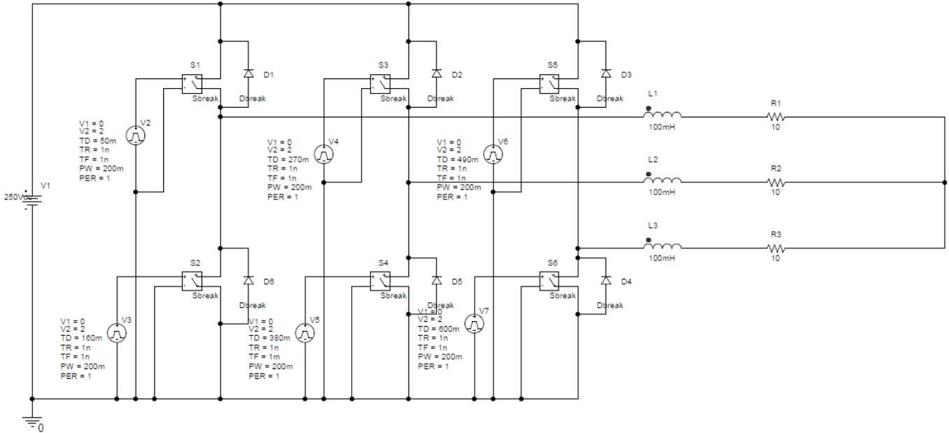
Fig. 21: Inverter circuit in PSpice used for co-simulation.
