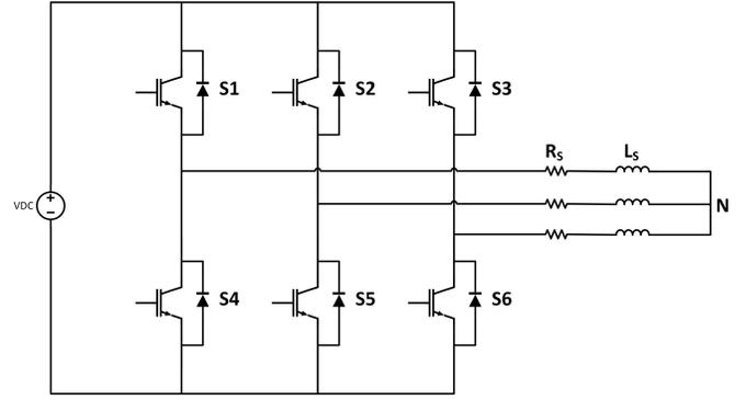
Fig. 10: Three-phase inverter
