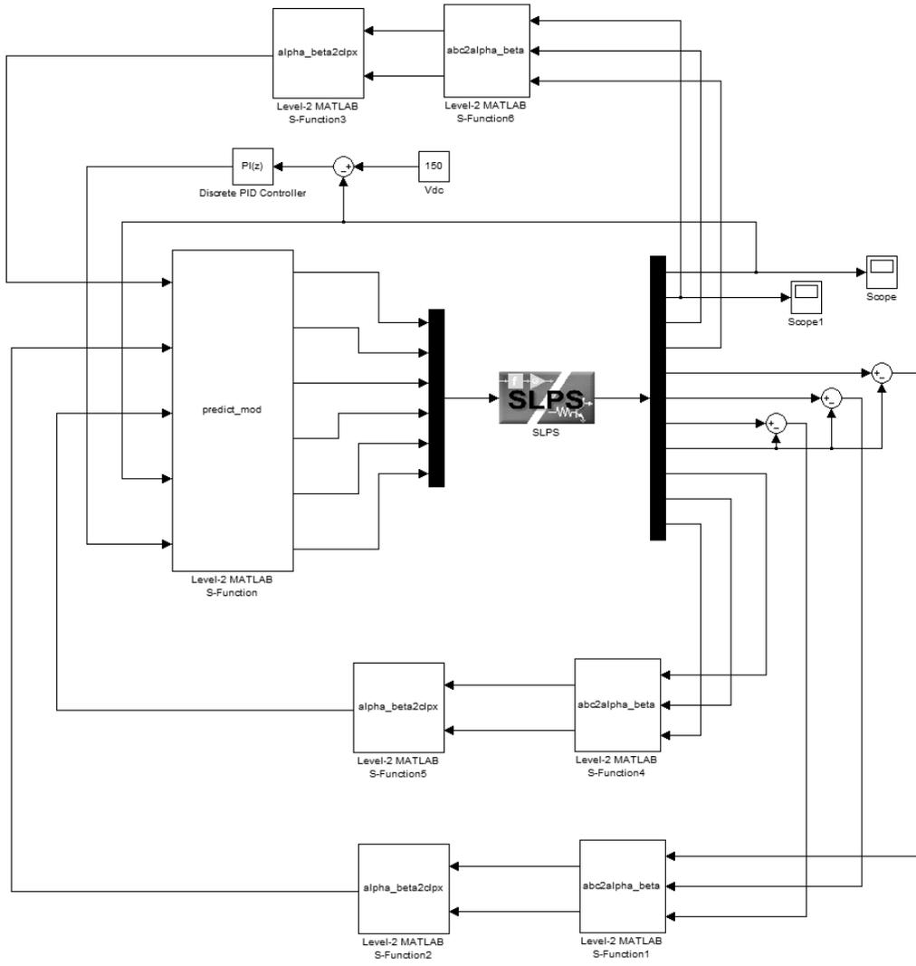
Fig. 17: Simulation of predictive control for the three-phase rectifier.
