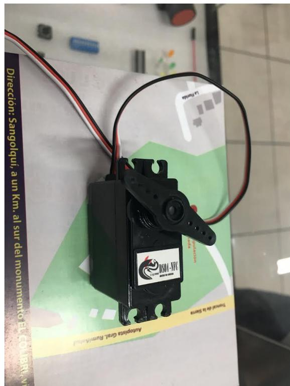
Figura 1-41 Servomotor Hi TEC HS 311
