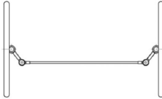
*Figure 65 Track Rod Mechanism Neutral Steer (Archibald, 2016)*
