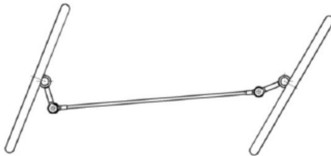
*Figure 66 Track Rod Mechanism 30 degrees Steer (Archibald, 2016)*
