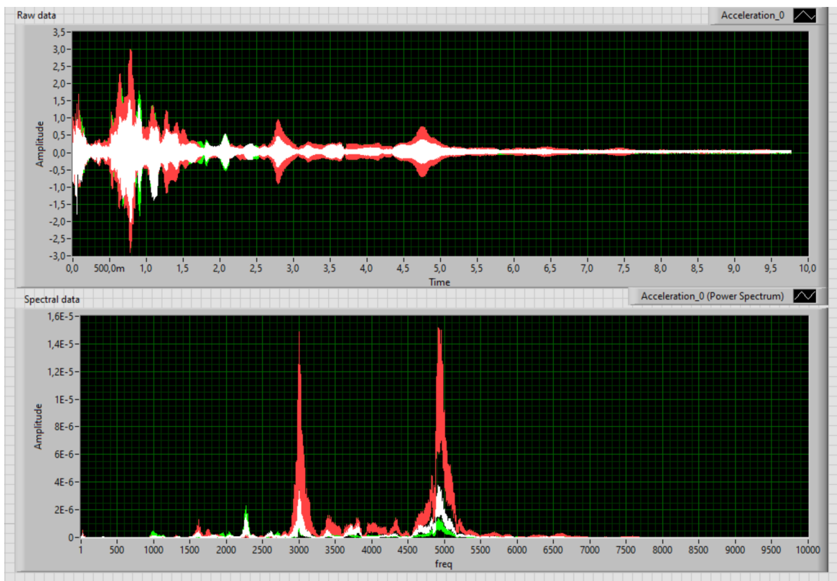
Figure 55. Raw and Spectral plot for the first set 1 Hz to 10 kHz from LabView number 1
