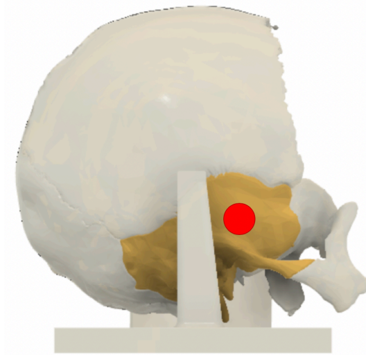
Figure 36. Location of the BC headphone right transducer.
