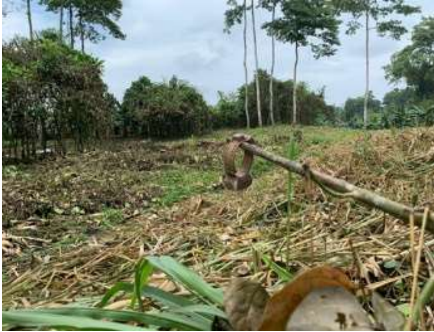
Figure 5: The image shows the testing for the collar to assure adequate signal strength and GPS point emission.
