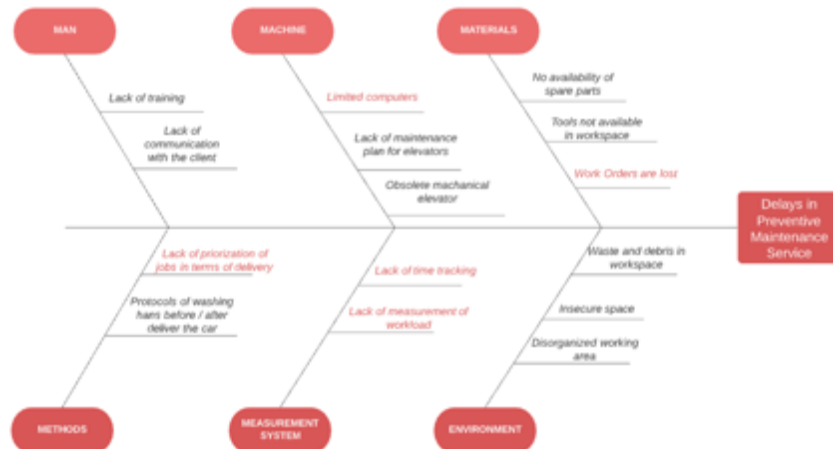
Figure 5: Cause and Effect Diagram for delays in preventive maintenance service.
