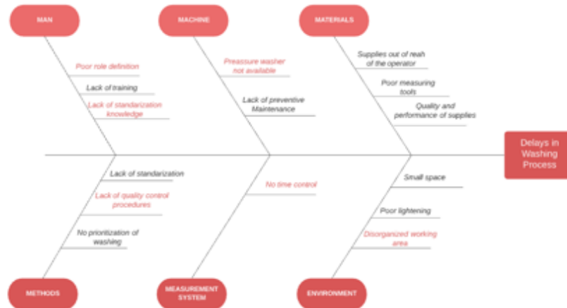
Figure 4: Cause and Effect Diagram for delays in washing process.
