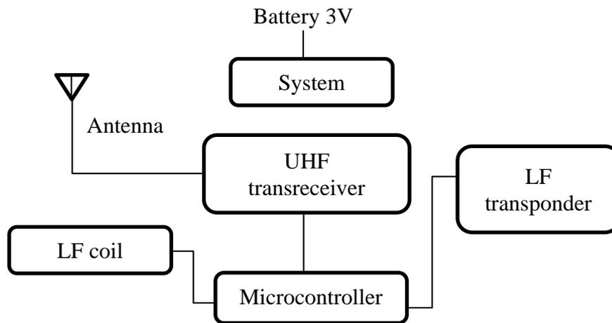
Figure 8. Key fob schematic
