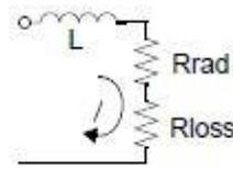
Figure 3. Equivalent loop antenna circuit
