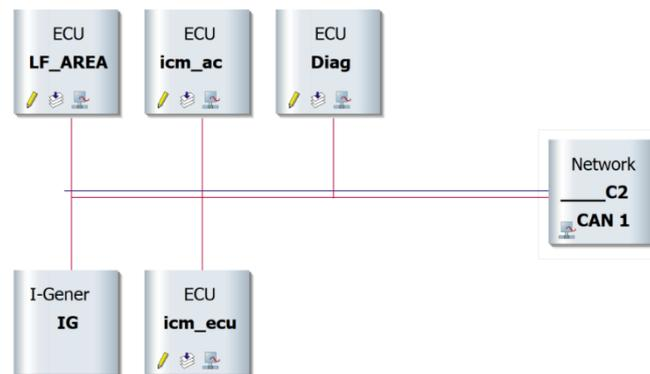
Figure 9. CAN connection Vector interface
