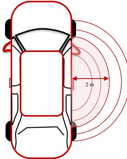
Figure 4. Car coverage magnetic field
