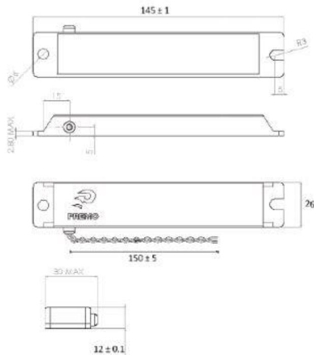
Figure 1. Car door mounted antenna
