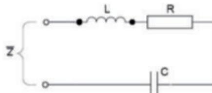
Figure 2. Car door antenna electrical diagram
