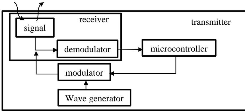
Figure 28. Key side schematic
