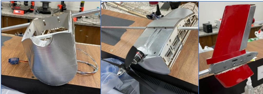
*Figure 19 3D printed components, wing aluminum tube and tail tube assembly*
