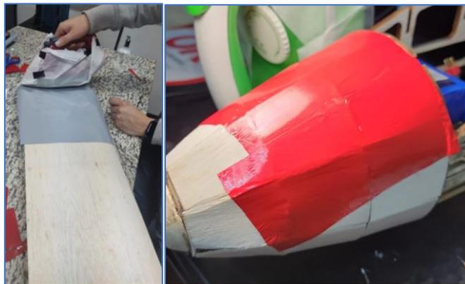
*Figure 16 Monokote coating process*
