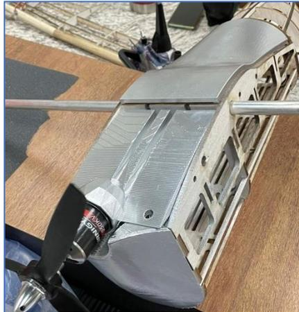
*Figure 41 Fuselage with 3D pieces*
