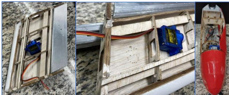
*Figure 14 Electronics components incorporation process*
