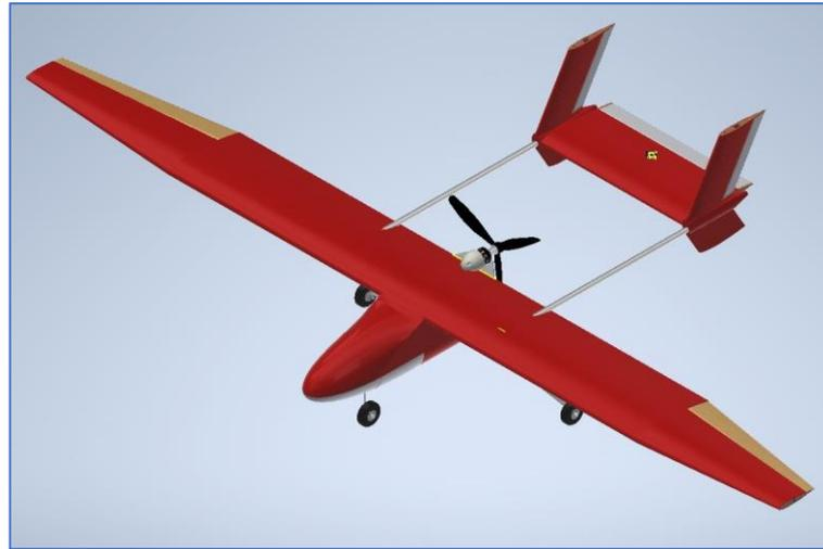
*Figure 40 CAD MK3 Assembly*
