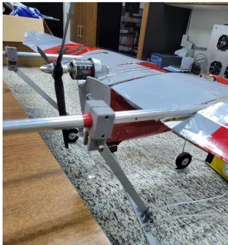
*Figure 44 Tail support from the landing gear*
