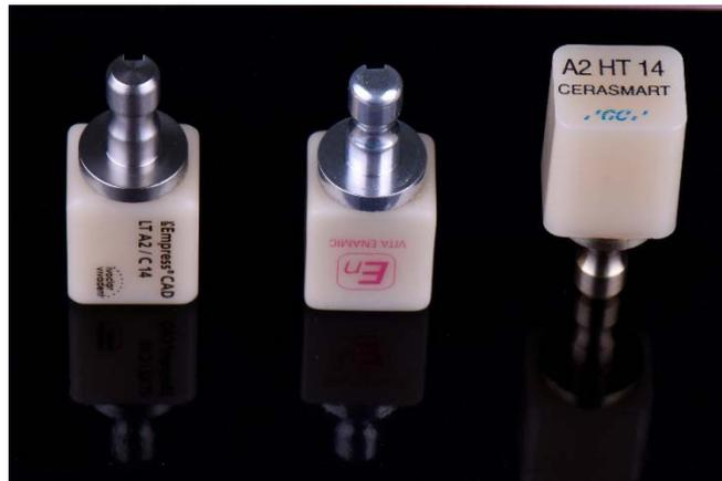
**Figura 1: Materiales empleados: Empress Cad, Vita Enamic, Cerasmart**
