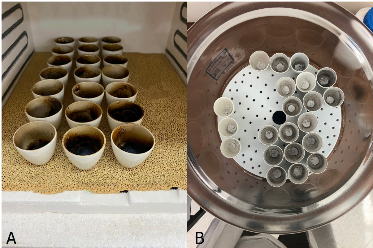
Figure 7. Ash test for samples of R. palmarum , three repetitions each. A: preheated samples before entering the muffle furnace, B: chilled samples after muffle furnace.
