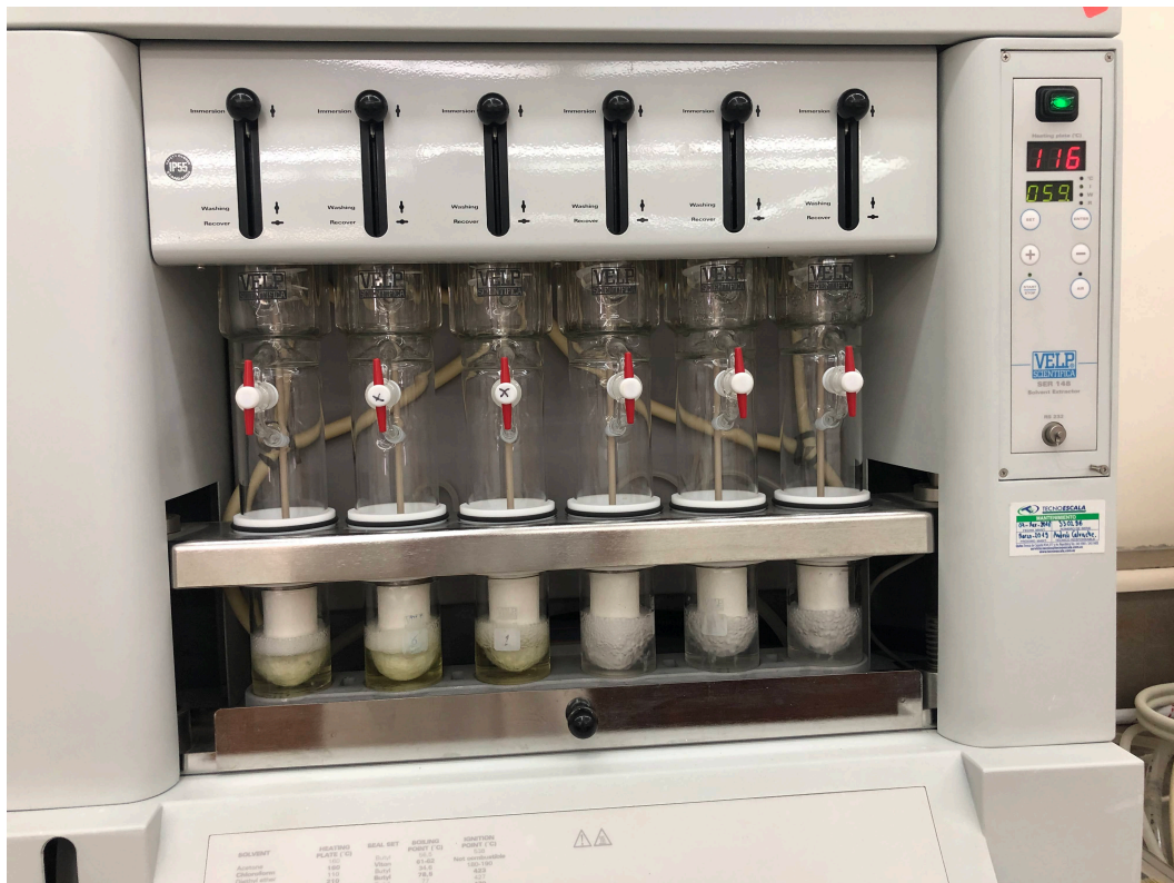
Figure 6. Fat test for two samples (8 and Cot, see Table 1) with three repetitions each. Start of immersion step.
