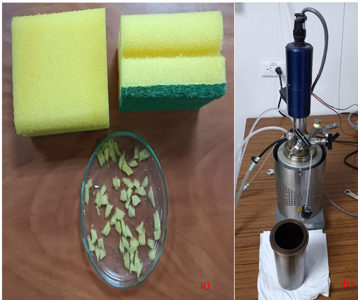
Figure 1: a) Pictures of PU foams and flakes used for depolymerization process, and b) reactor setup used for PU methanolysis
