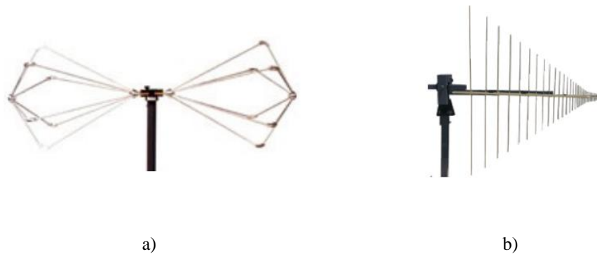
Fig. 2.6 Broadband antennas for EMC measurements: (a) Biconical antenna b) Log-Periodic antenna.
