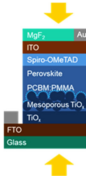
Figure 3. 7: Schematic structure of the perovskite solar cells using ITO. Reproduced from (Bett, et al., 2019)
