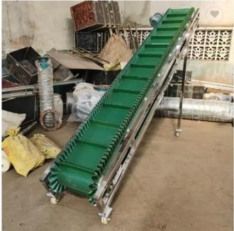
Large dip Angle feeding belt conveyor Dryer feeding belt conveyor
