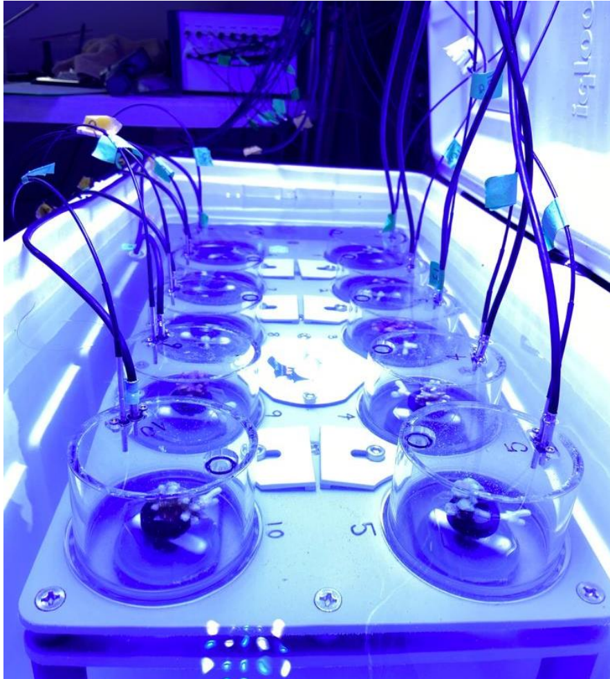
Figure 1. Respirometry system. Ten acrylic chambers (nine for species' individuals, one as control) measuring O 2 consumption rates and water temperature by using two probes. These probes were connected to a computer in order to record and visualize the measurements in real time.
