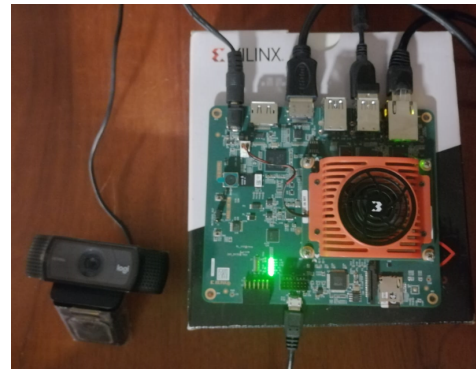
Fig. 4. Hardware Setup for the KV260.
