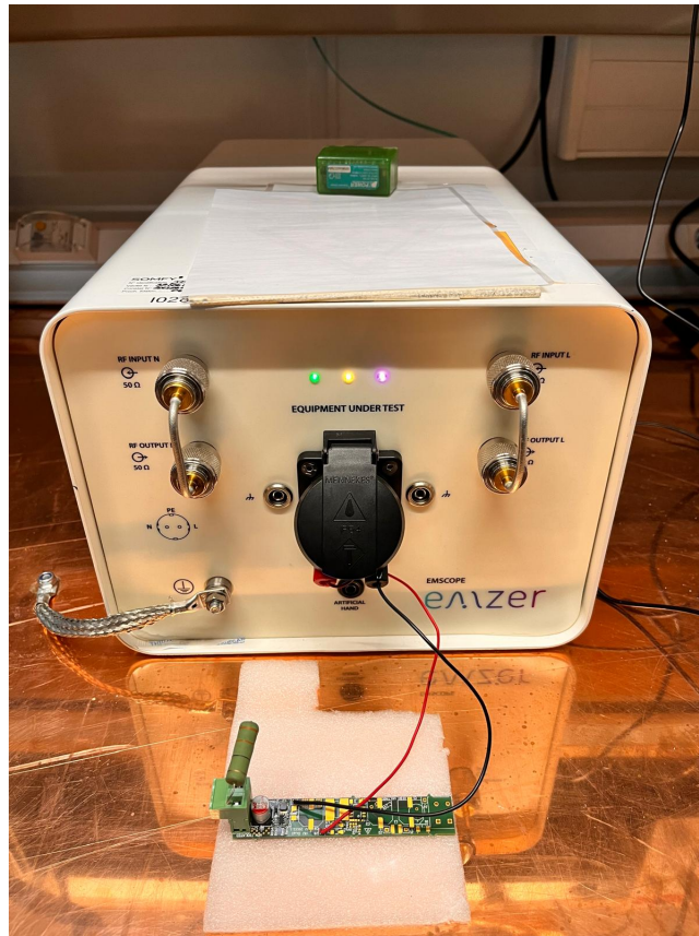
Figure 4.1: Generation of the measure data with EMSCOPE and connection of low voltage buck converter.
