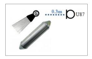
Figura N. 18 Güiro mic setup
