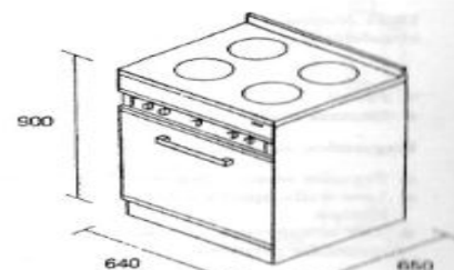
y Medium-duty oven range, 84 litres with four radiant rings, 8 kW rating
