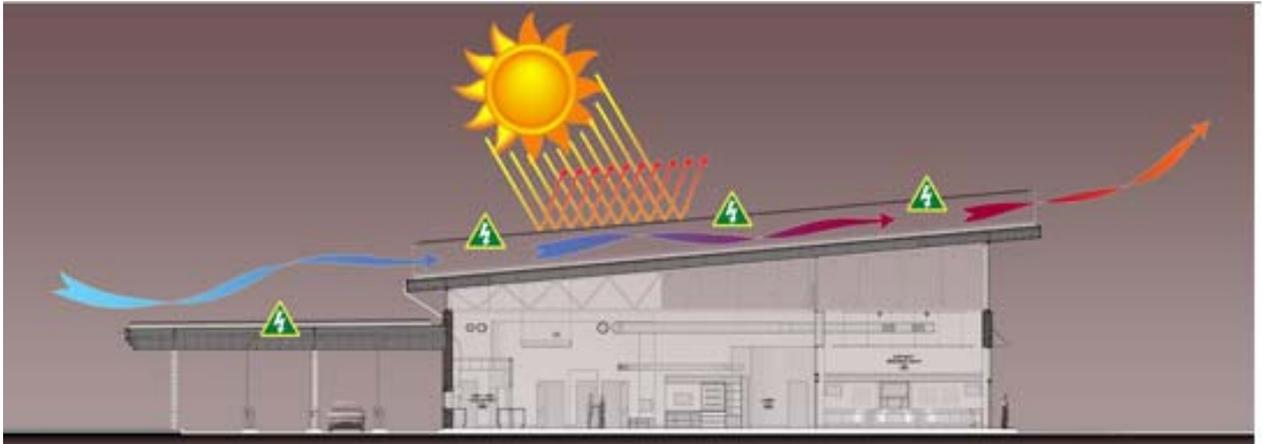
*Figura 3. Sistema de doble techo (Straughn Trout Architects, 2015)*
