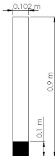
Figure 1. Dimensions of the simulated fluidized bed based on the experimental setup
