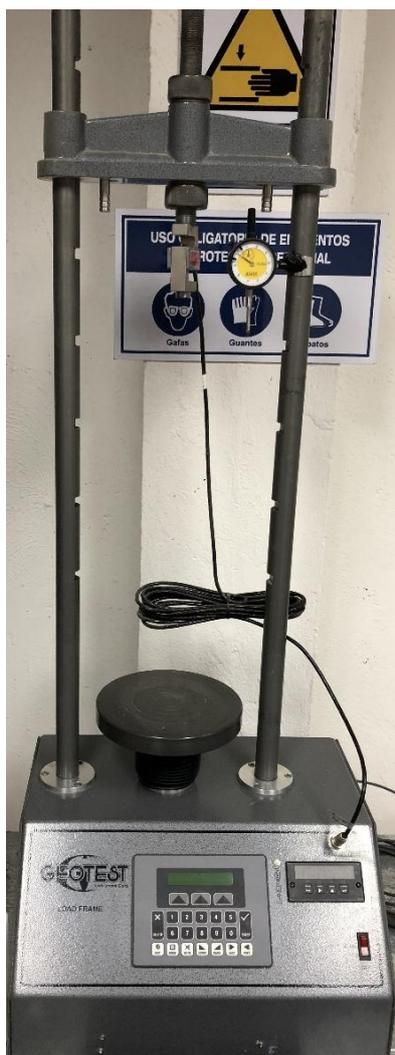
Figura A. 1: Marco de carga Geotest.
