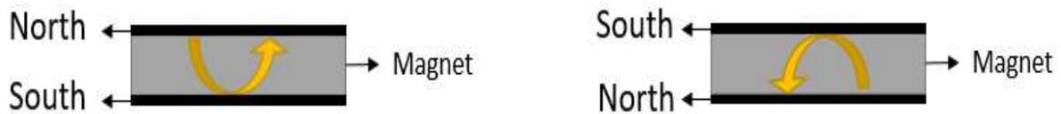
Figure 5: Two configurations of a magnet: North-South (NS) and South-North (SN) where “black layers” represent the poles.
