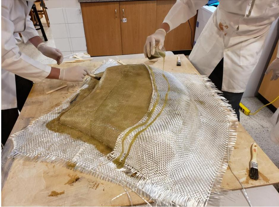
*Figure 36 Application of fiberglass*
