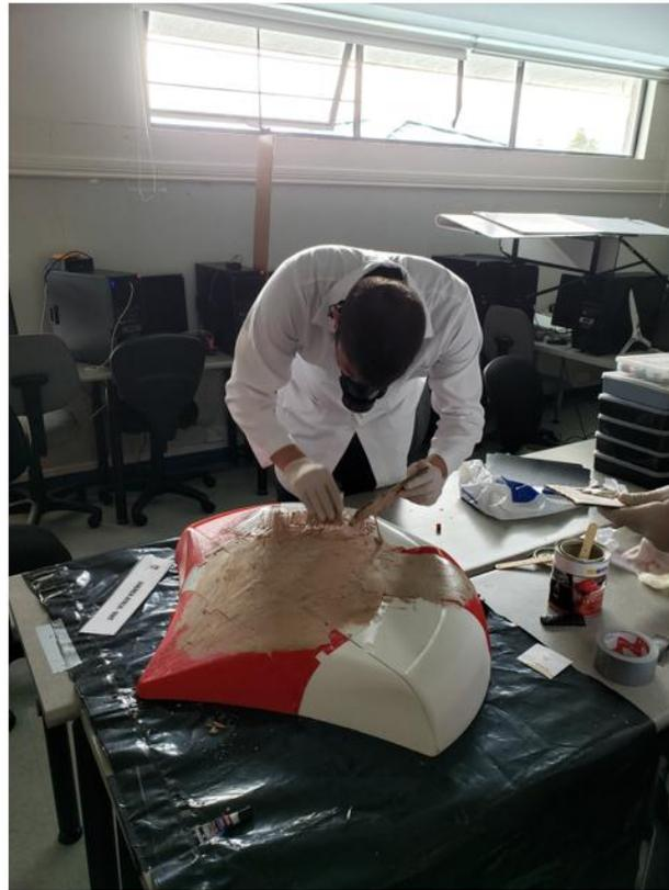
*Figure 32 application of filler over the cast*
