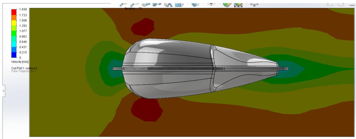
Figure 21 Cut plot velocity Stingray
