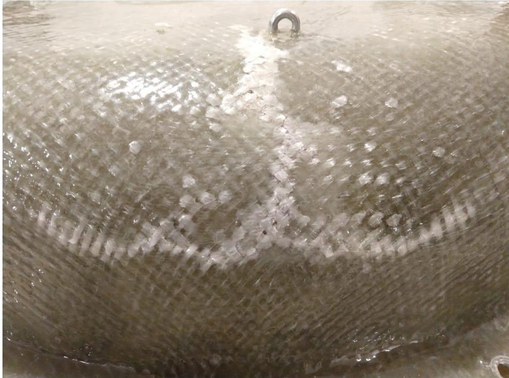
*Figure 51 crack in the hull (front)*
