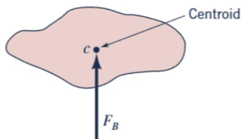
Figure 4 Center of buoyancy on a submerged body (Gerhart, Gerhart, & Hochstein, 2016)
