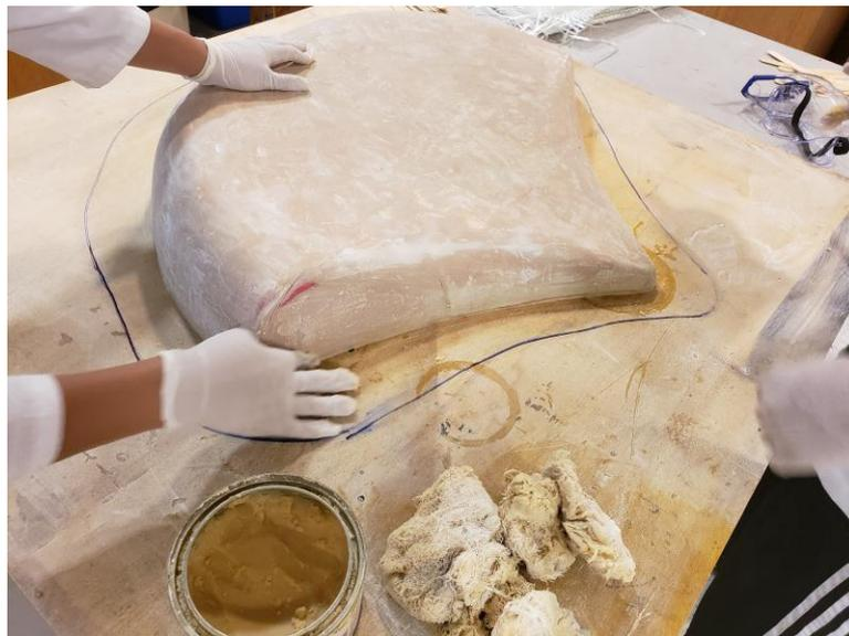
*Figure 35 covering of mold with grease*
