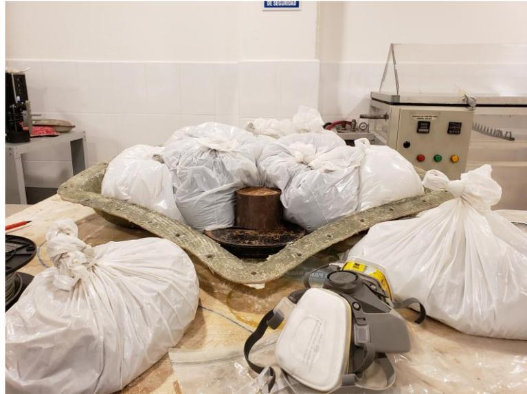
*Figure 48 neutral buoyancy weight distribution*
