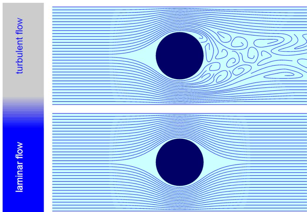
Figure 6 Comparison between laminar and turbulent Flow (Gerhart, Gerhart, & Hochstein, 2016)
