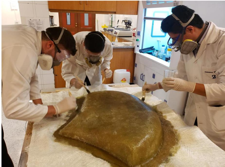
*Figure 37 Application of vinyl ester resin*
