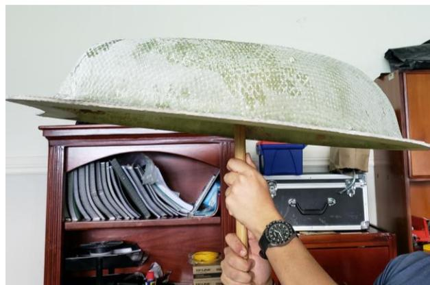
*Figure 43 Determination center of gravity*
