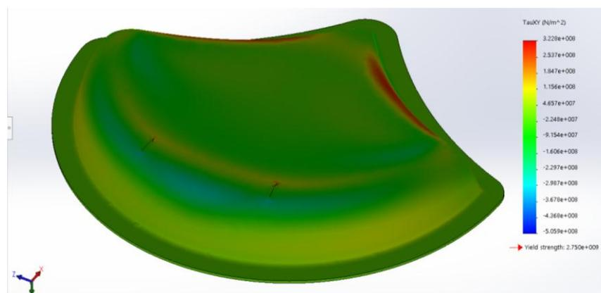
Figure 28 Shear stress in XY plane
