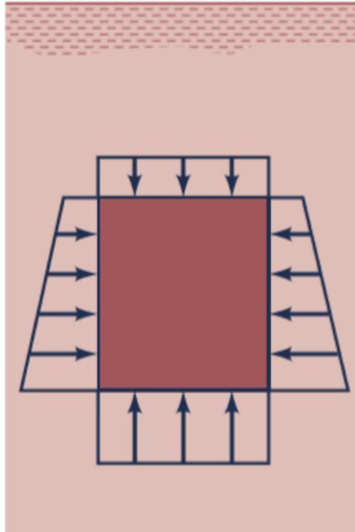
Figure 3 Pressure on a submerged body (Gerhart, Gerhart, & Hochstein, 2016)
