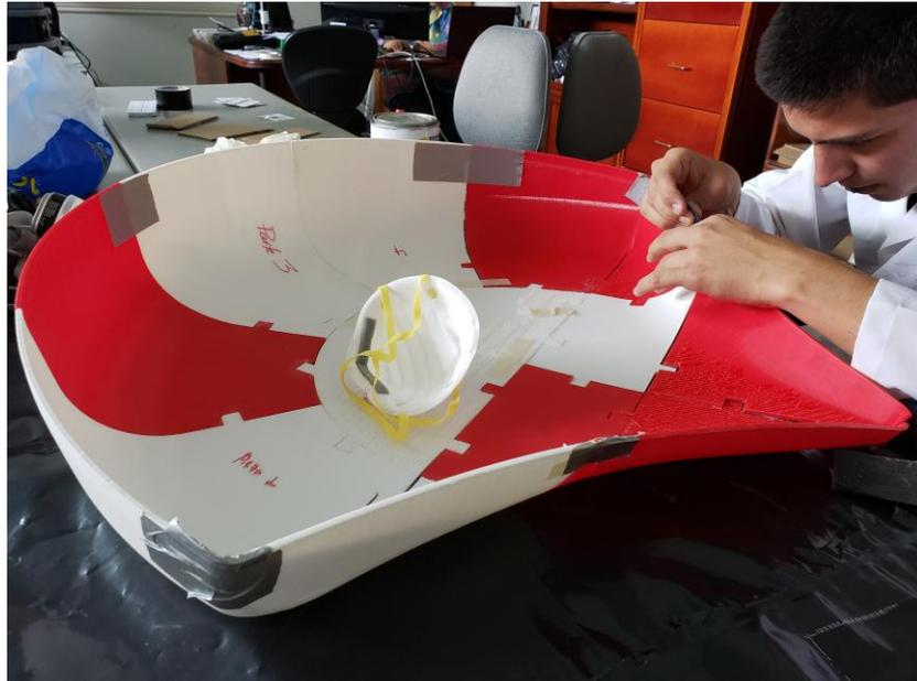
*Figure 30 Assembling of the 3D printed mold*
