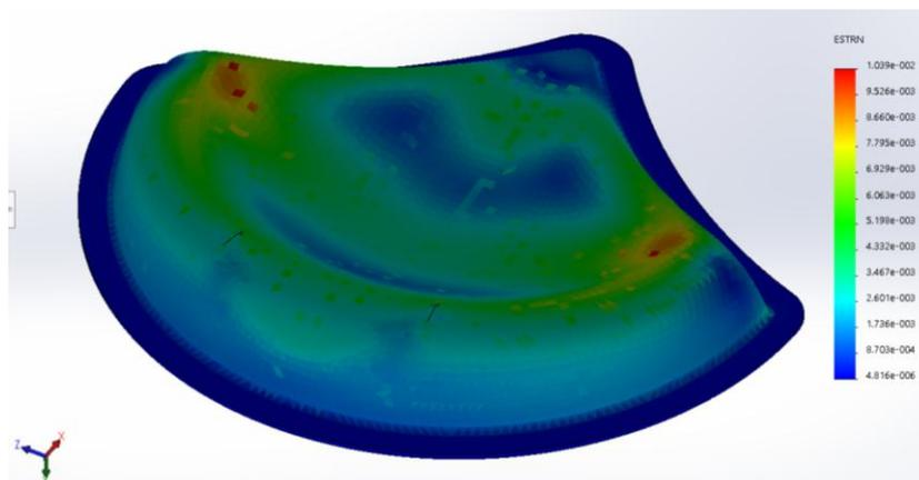
*Figure 24 Strain plot*
