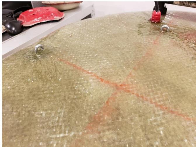
*Figure 47 cable anchors on the submarine*
