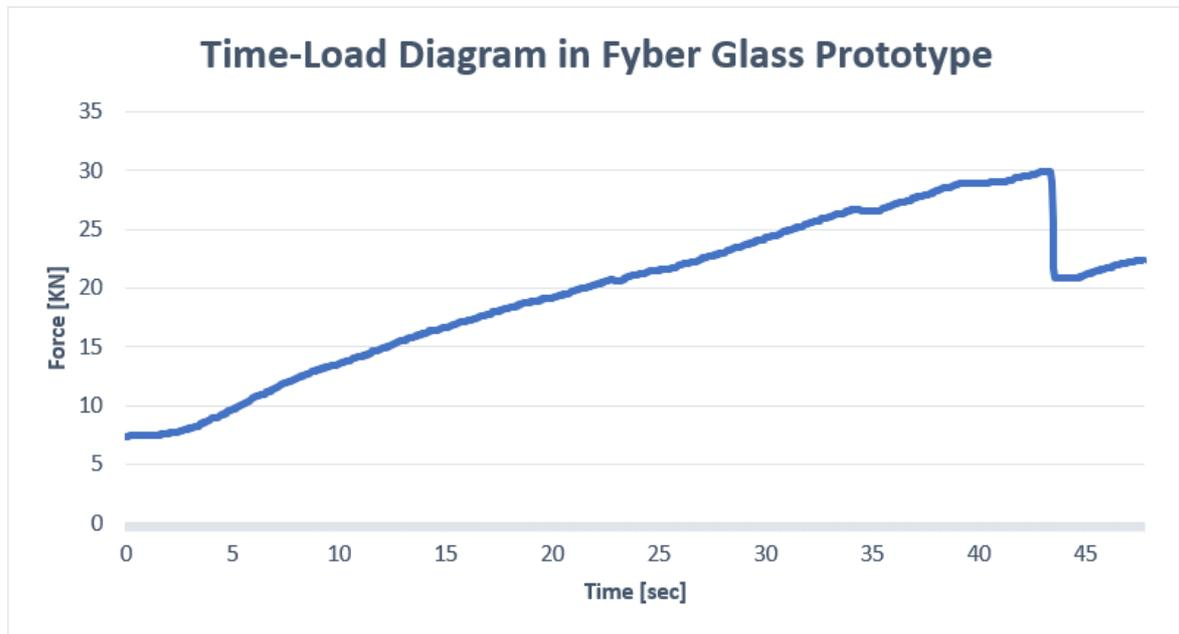
*Figure 16 Compression test results on prototype*
