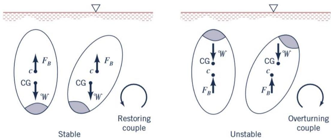
Figure 5 Stability of submerged bodies and restoring couples (Gerhart, Gerhart, & Hochstein, 2016)
