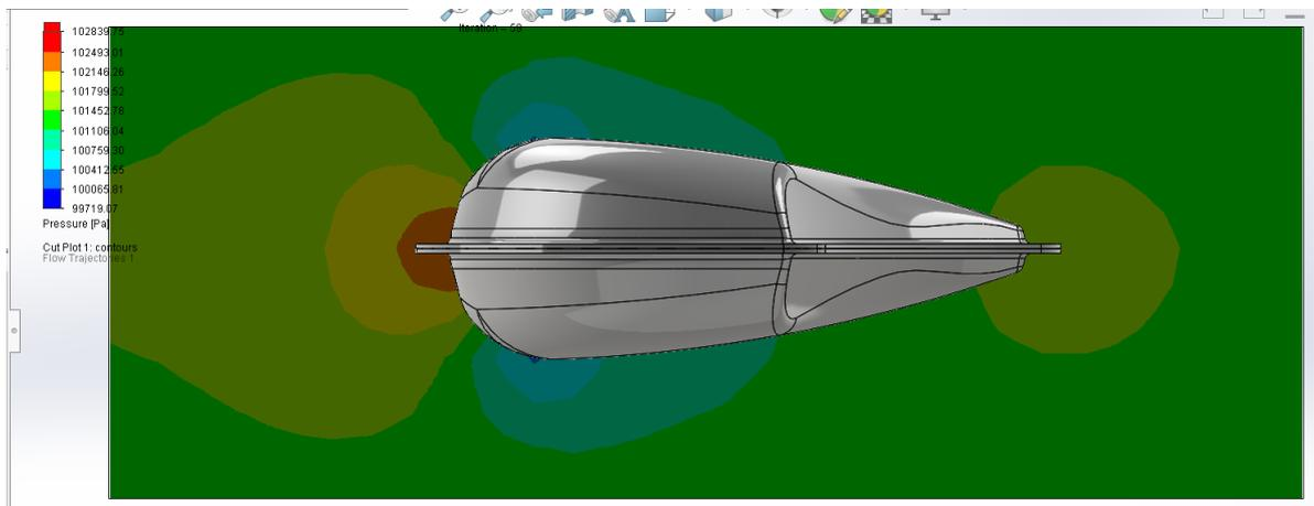
*Figure 19 cut plot pressures Stingray*
