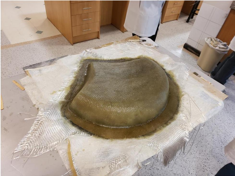
*Figure 38 hull result*
