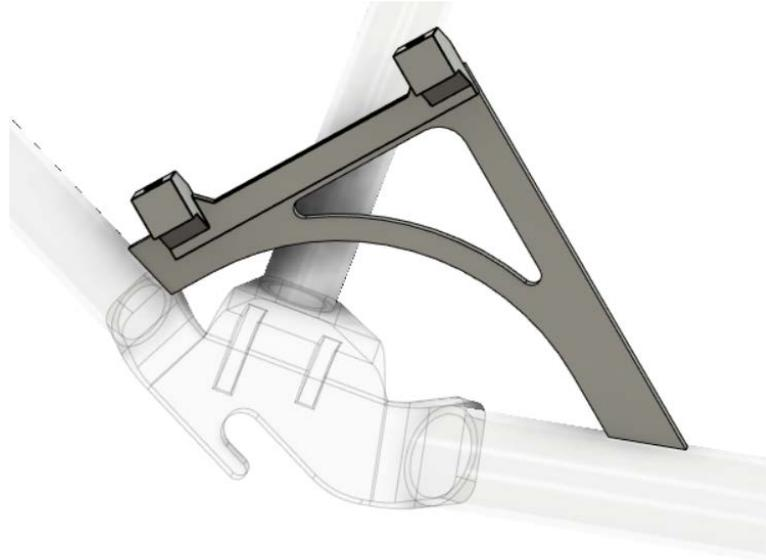
*Figure 51 Rear Wheel Caliper Mount*
