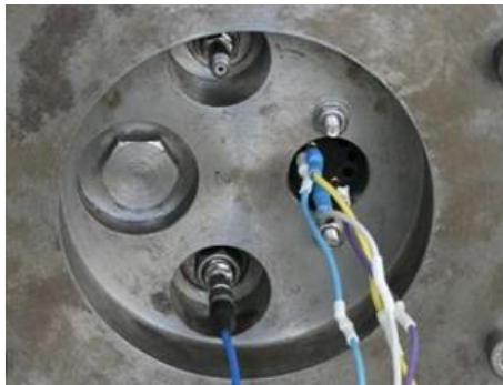
Figure 14: Connections between sensor and conditioning circuit.
