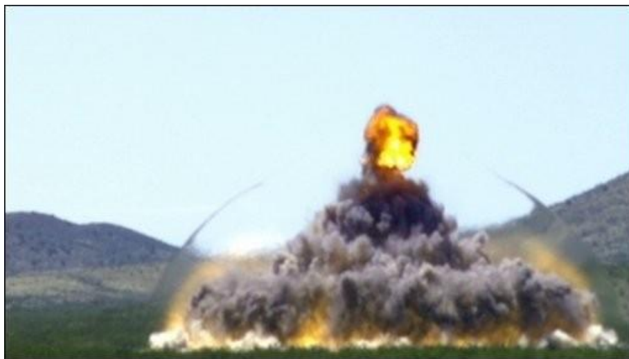
Figure 2: Picture of a blast wave with its typical spherical shape.[2]
