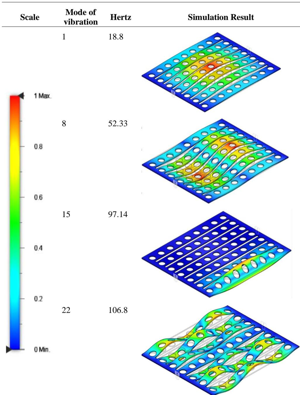
Results of Table 20 and table 21 seem to show Fusion 360 software recognize each row of the container as an individual beam. For this reason, the table below brings under vibration analysis to the individual beam. First four vibration modes of the single beam are represented in table 22.
