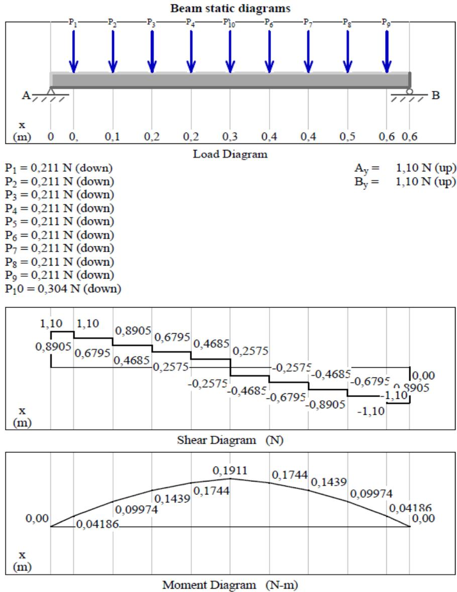
*Figure 11 Beam diagrams*
