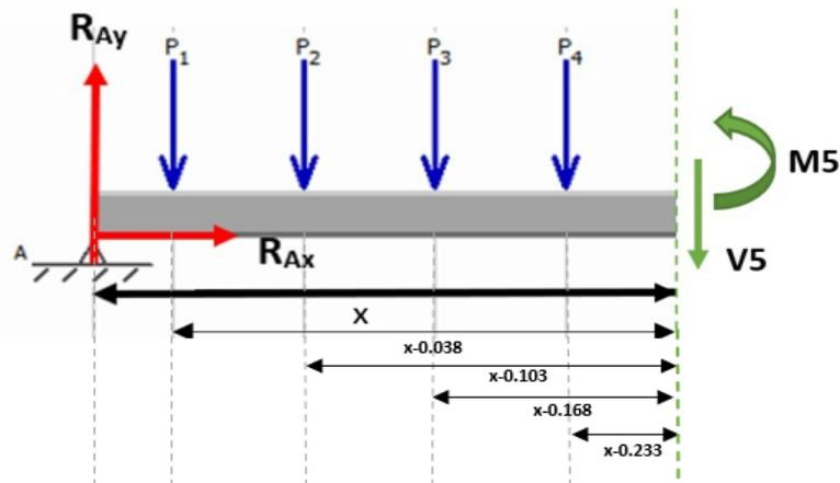
Figure 10 Cut section for the section method
