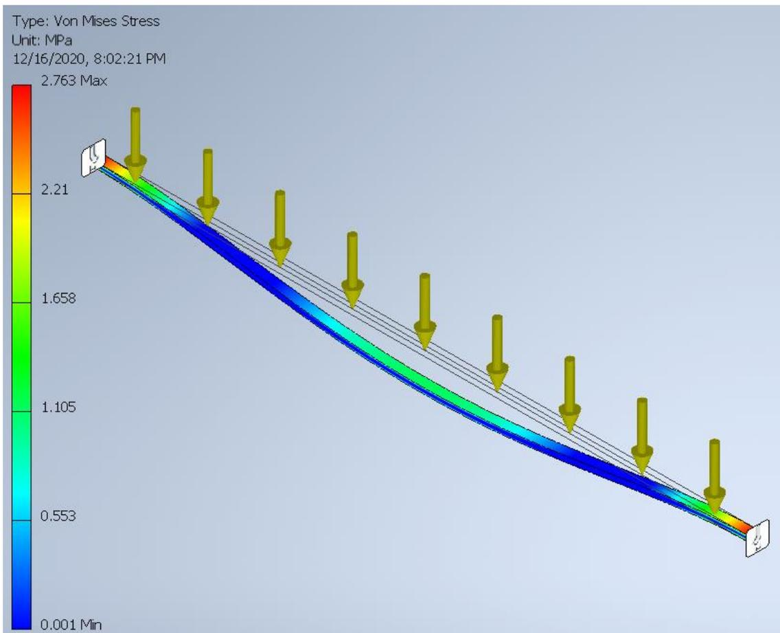
Figure 20 Maximum stress of the critical zone embedment
