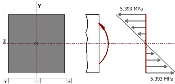
Figure 14 Normal stress calculated with MDSolids Software
