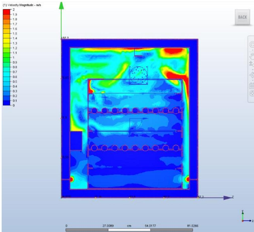
Figure 33 Front view first design CFD heat and fluid simulation
