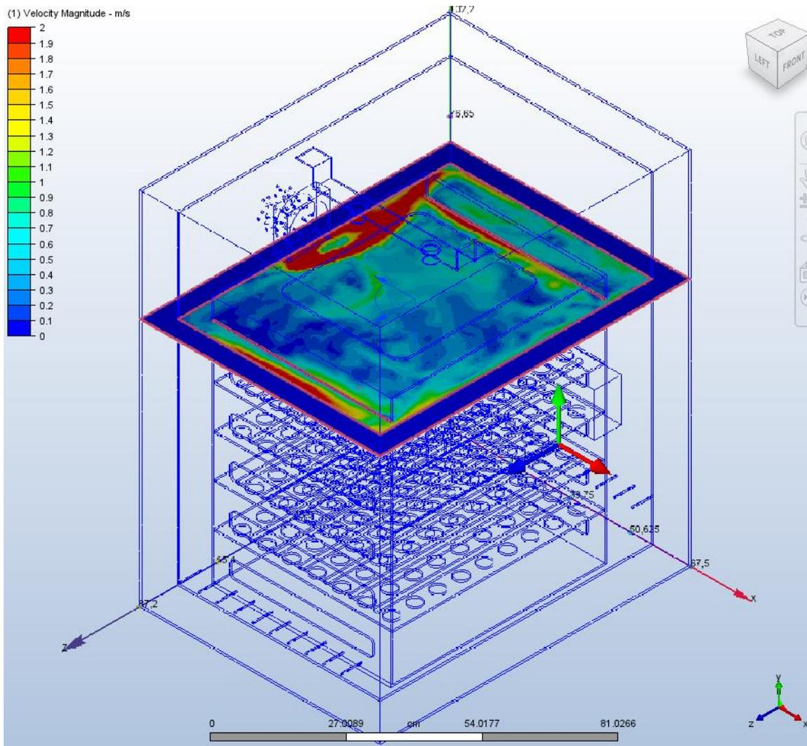
Figure 31 Offset plane first design CFD heat and fluid simulation
