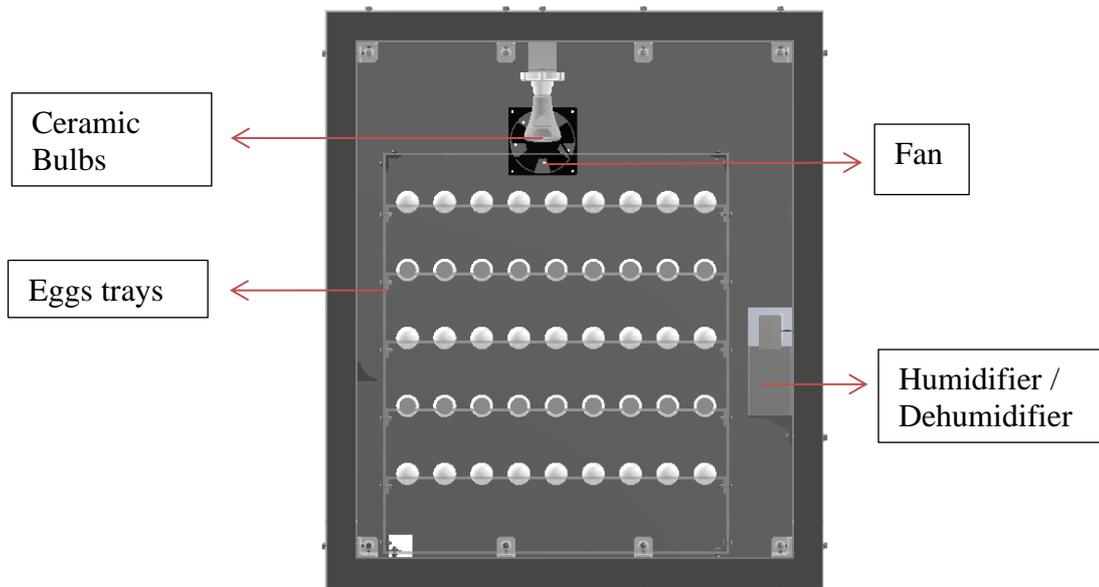
*Figure 3 Visual incubator representation with principal components*
