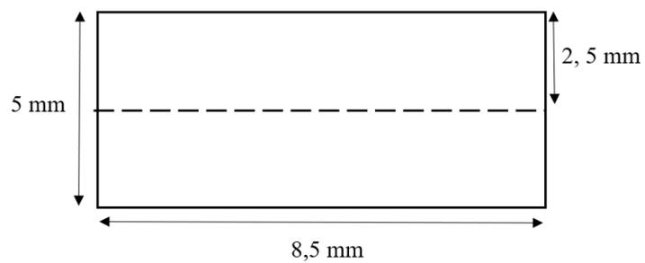
*Figure 5 cross sectional area of the critical beam to analyze*
