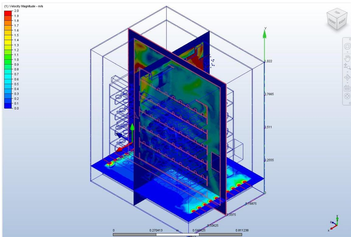
Figure 36 multi offset planes view second design CFD heat and fluid simulation
