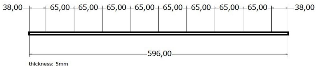
Figure 9 Dimensions of the geometry of the beam
