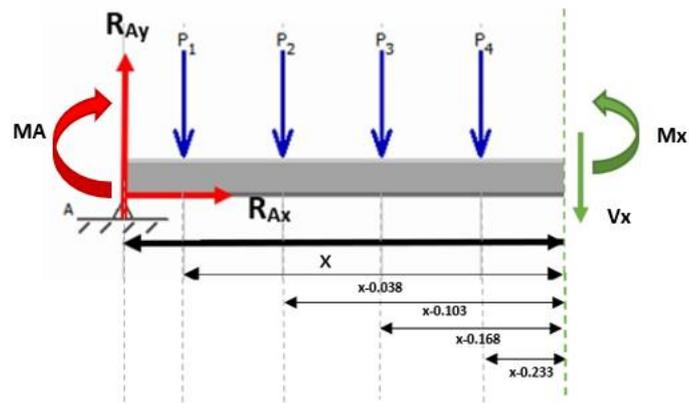
Figure 19 Embedment section cutter for the section method
