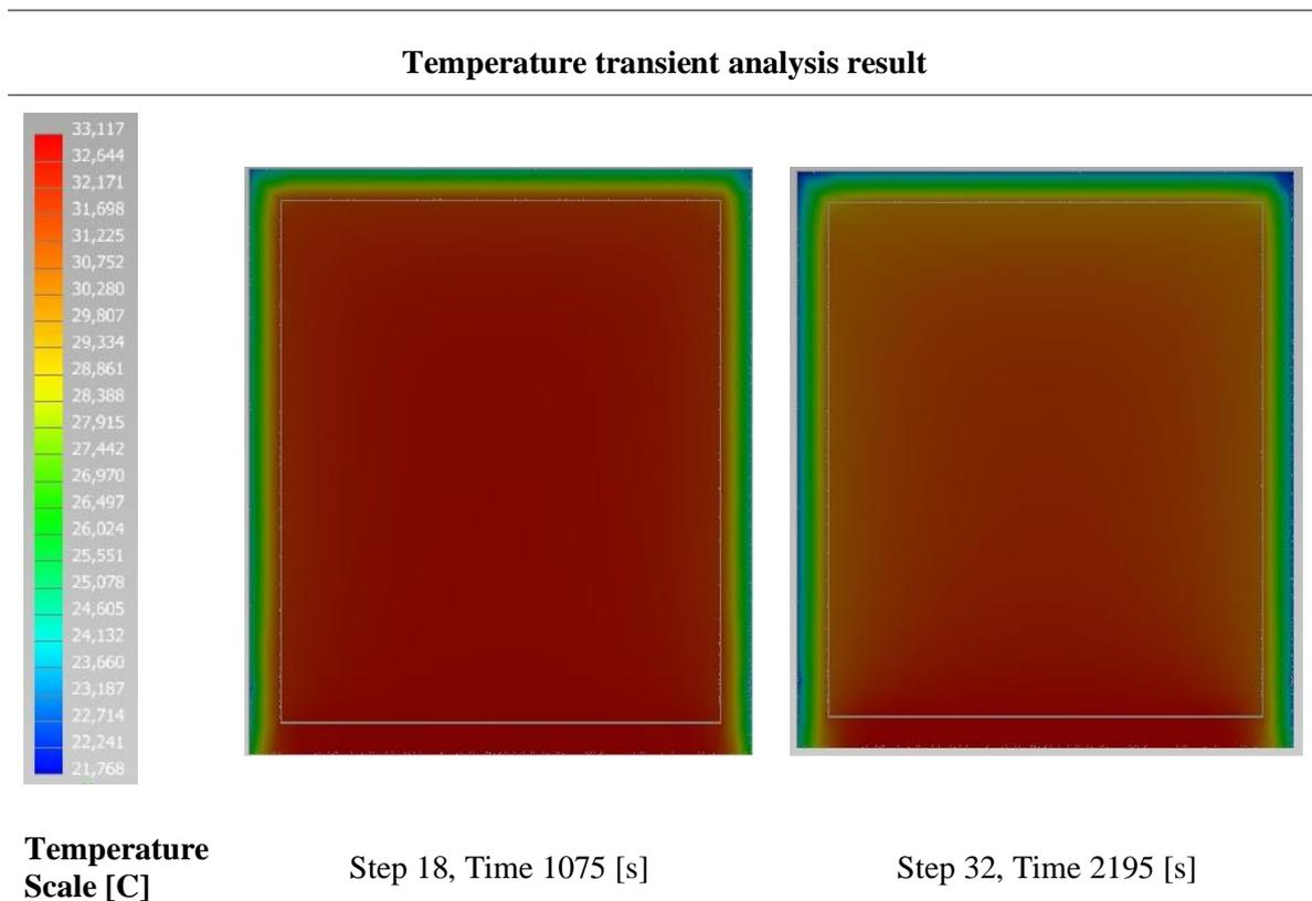
Figure 27 presents temperature variation caused by vents. It can be inferred that these cavities will not cause mayor temperature losses on the system.
