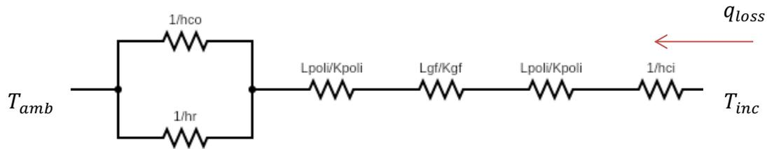
Figure 26 Representative resistance circuit for heat flow through walls
