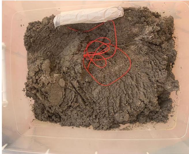
*Figure 28 Sand container with data logger and thermocouple*
