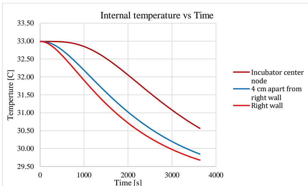
From table 37 it can be observed that at the sensor location, blue line, a degree Celsius is lost in 1155 seconds. In contrast, incubator center point takes 2115 seconds to decrease its temperature in the same amount. Schematic representations of temperature loss in function of time can be appreciated on table 38. It can be observed how outer incubator components reduce their temperature faster.
