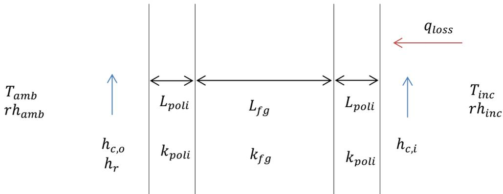
Figure 25 One dimensional heat flow through composite wall diagram
