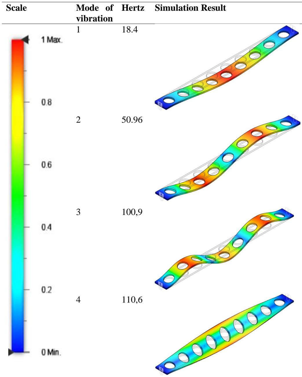
Stiffening an element requires usually a more rigid material. Seeking the mitigation of the first modes of vibration (which are the most critical), it is designed an extra component with higher rigidity. Since the future location of the incubator has a high relative humidity, avoid corrosive materials is a requirement. Organic materials are another restriction due to its
