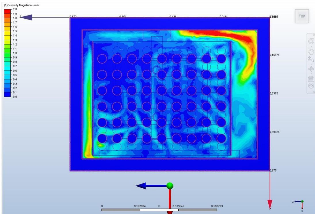
Figure 38 Top view second design CFD heat and fluid simulation
