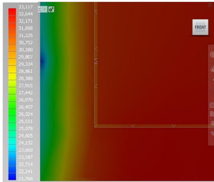
Figure 27 Temperature variation in vents transient simulation
