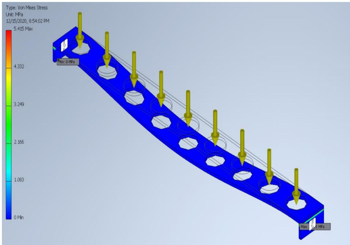
Figure 18 maximum stress of the beam
