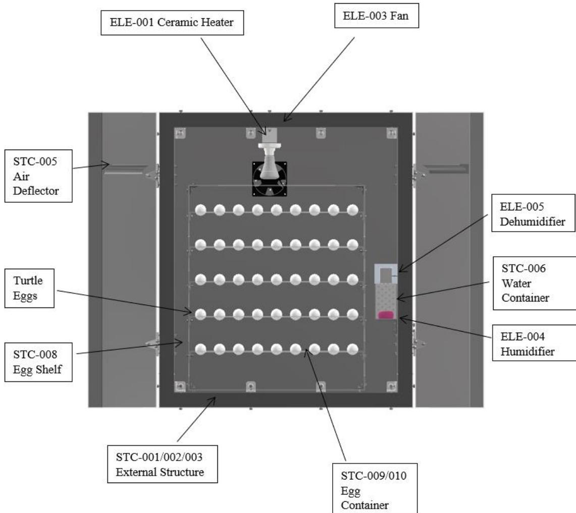
*Figure 39 Assembly with labels*
