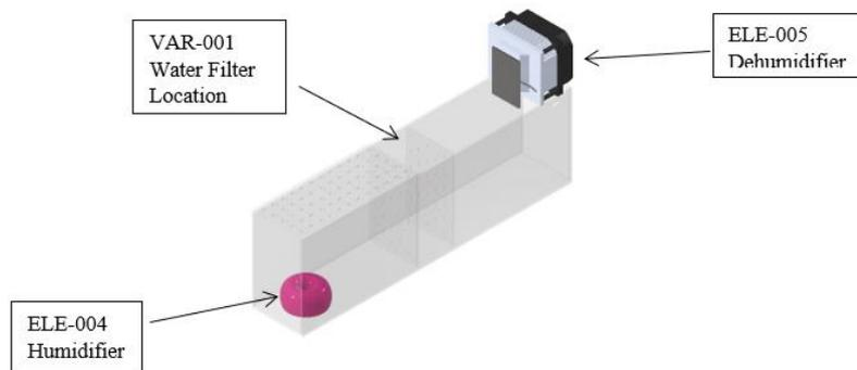
*Figure 40 Water container assembly*
