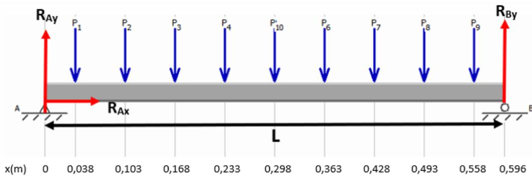
Figure 8 Free body diagram of the beam
