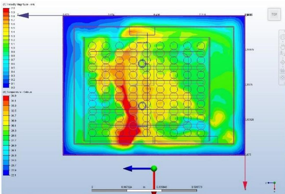
Figure 35 Top view second design CFD heat and fluid simulation
