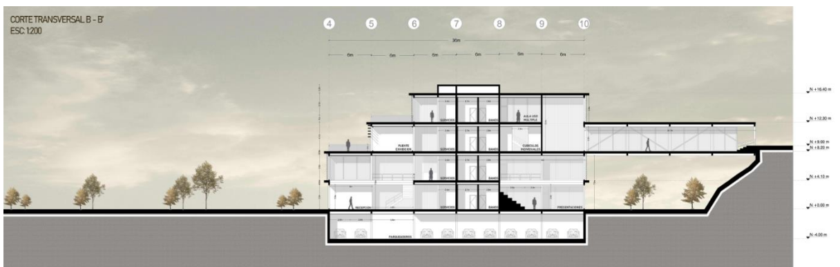
Figura #25. Corte Transversal B – B’
