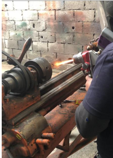
Figure 3 HAp addition by thermal spray HVOF process
