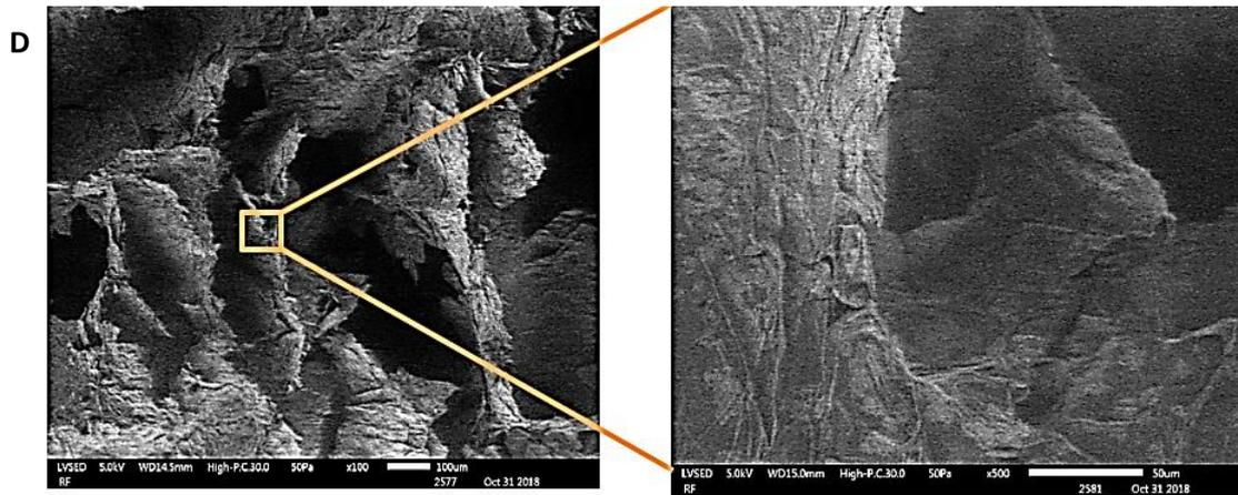
*Figure 14. Scanning electron micrographs of different cacao-mesocarp scaffolds. The formulations chosen from the DOE were: A) central point (58.90 [%w/w] cellulose, 14.48 [%w/w] lignin); B) Scaffold 5 (45.78 [%w/w] cellulose, 22.01 [%w/w] lignin); C) Scaffold 25 (59.94 [%w/w] cellulose, 21.91 [%w/w] lignin); D) Scaffold 28 (64.57 [%w/w] cellulose, 15.68 [%w/w] lignin). The images were taken at 100X (left) and 500X (right).*
