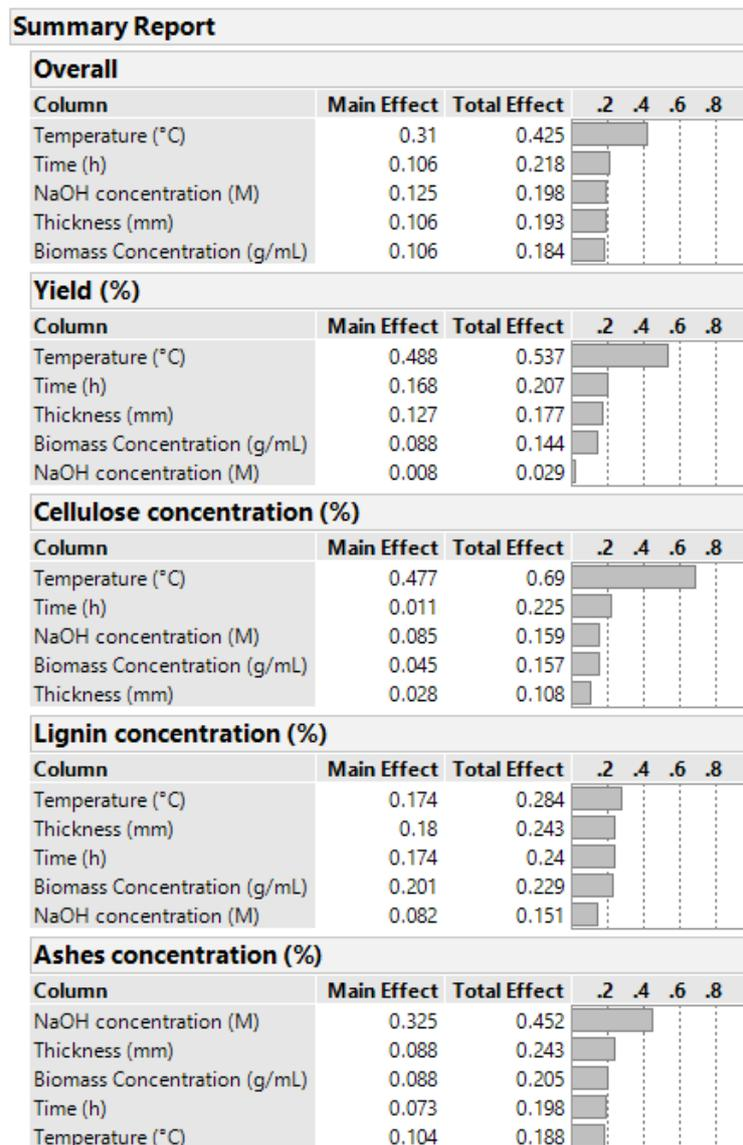
Figure 9. Level of influence of each input variable (Temperature, time, NaOH concentration, thickness, biomass concentration) in the experiment model.
