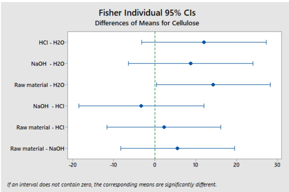
Figure 21. Fisher plot with 95% of confidence interval. Analysis to determine the differences of means for Cellulose in each treatment.
