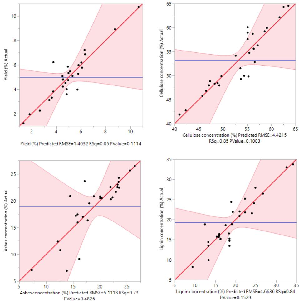
Figure 8. Variability of the responses according to output variables (lignin, cellulose, ashes and yield) black dots represent the data for the model.
