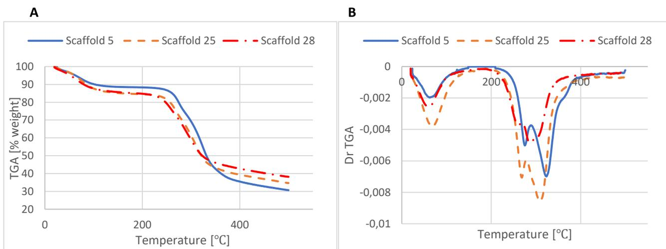
Figure 11. Thermal analysis of scaffold 5 ( $45.78$  [%w/w] cellulose,  $22.01$  [%w/w] lignin); scaffold 25 ( $59.94$  [%w/w] cellulose,  $21.91$  [%w/w] lignin); scaffold 28 ( $64.57$  [%w/w] cellulose,  $15.68$  [%w/w] lignin). A) Thermogravimetric (TGA) curve, B) Differential thermogravimetric (DTG).
