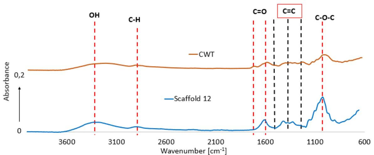
Figure 12. FT-IR spectrum of one central point of the model, cellulose content: 58.90 [%w/w]; lignin content: 14.48 [%w/w], compared with the spectrum of the cacao without treatment (CWT), red bands represent characteristic peaks of cellulose and black bands represent the characteristic peaks of lignin.
