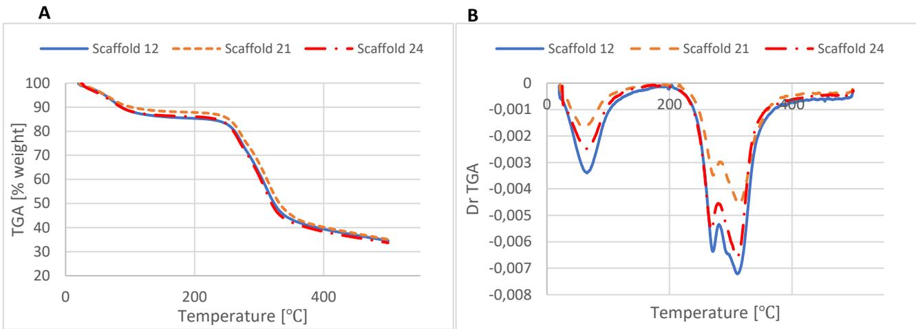
Figure 10. Thermal analysis of central points of experimental model (scaffolds 12, 21 and 24 with cellulose content: 58.90 [%w/w]; lignin content: 14.48 [%w/w]) A) Thermogravimetric (TGA) curve, B) Differential thermogravimetric (DTG).
