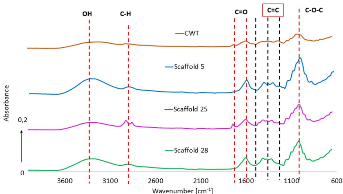
Figure 13. FT-IR spectra of scaffold 5 (45.78 [%w/w] cellulose, 22.01 [%w/w] lignin); scaffold 25 (59.94 [%w/w] cellulose, 21.91 [%w/w] lignin); scaffold 28 (64.57 [%w/w] cellulose, 15.68 [%w/w] lignin), compared with the spectrum of the cocoa without treatment (CWT), red bands represent characteristic peaks of cellulose and black bands represent the characteristic peaks of lignin.
