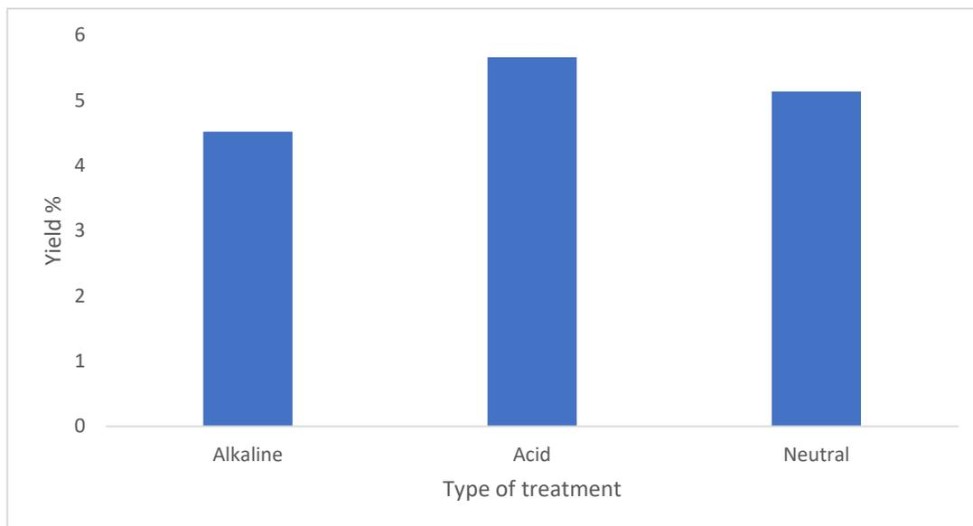
*Figure 3. YPP of each treatment applied to the mesocarp, acid treatment presents the highest YPP (analysis without repetitions).*
