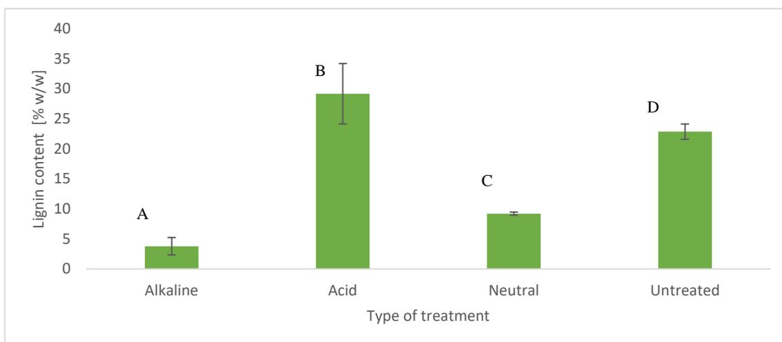
Figure 4. Effect of different treatments (alkaline, acid and neutral) on the content of lignin on scaffolds obtained from the mesocarp of cacao CCN-51 pod shell. **Bars** with the same letter represent the treatments with no significant differences, while different letters represent treatments that were significantly different ( $p < 0.05$ ).
