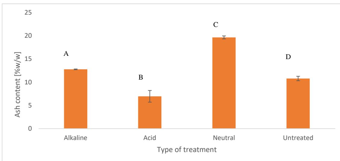
Figure 6. Effect of different treatments (alkaline, acid and neutral) on the ash content on scaffolds obtained from the mesocarp of cacao CCN-51 pod shell. **Bars** with the same letter represent the treatments with no significant differences, while different letters represent treatments that were significantly different ( $p < 0.05$ ).
