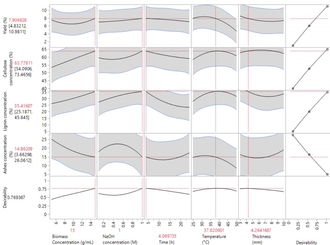
Figure 7. DOE prediction profiles of output variables as functions of input variables, according to experimental data. Vertical dotted red lines show the values of each input variable that optimize the desirable output variables.
