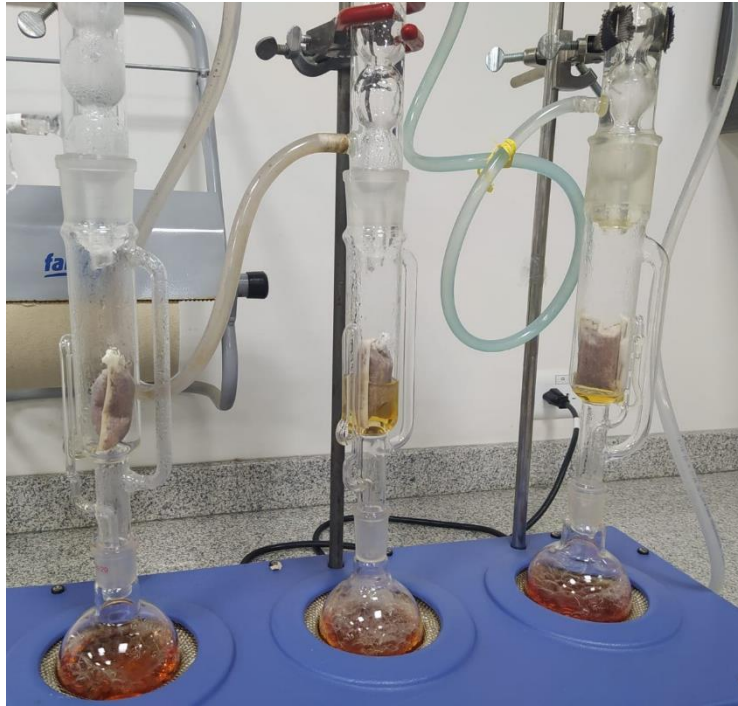
Figure 16: Soxhlet extraction from avocado seed in water done in triplicate (Hour number 5 of extraction).
