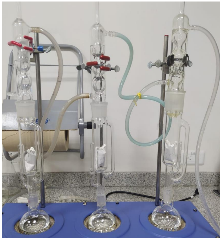
Figure 13: Soxhlet extraction from avocado seed in water done in triplicate (Start of extraction).
