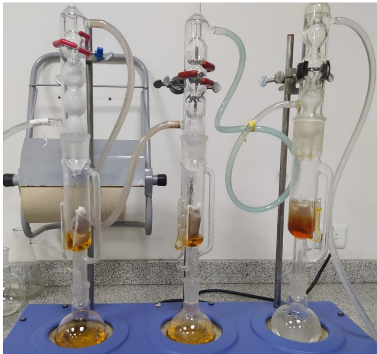
Figure 14: Soxhlet extraction from avocado seed in water done in triplicate (Hour number 2 of extraction).
