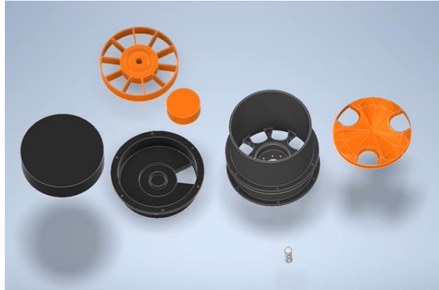
Figure 54: complete set of designed pieces of the seed distribution system.
