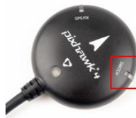
Figure 3: GPS module. (Safety Switch/LED)
