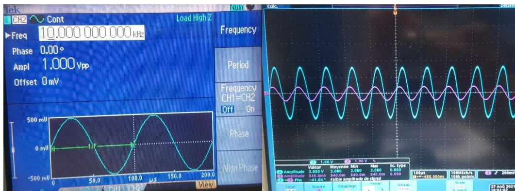
Figure 42. Waveforms for input and output signal when V_{in\ pk-pk}=1[V] at f=10 [kHz].
