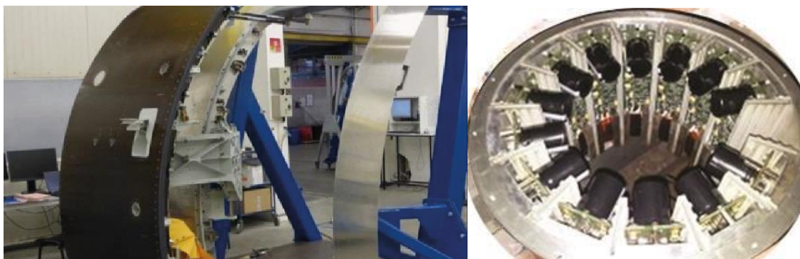
Figure 1. At the left - NEXGED project for Latécoère, electric piloting of an aircraft door. At the right - Powerful electric motor developed by Novatem. (NOVATEM SA, 2020)
