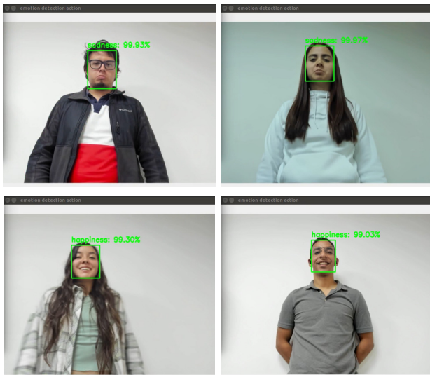
Fig. 8: Real-time prediction examples, a green frame is drawn around the face, indicating the classified expression and its corresponding prediction confidence value.
