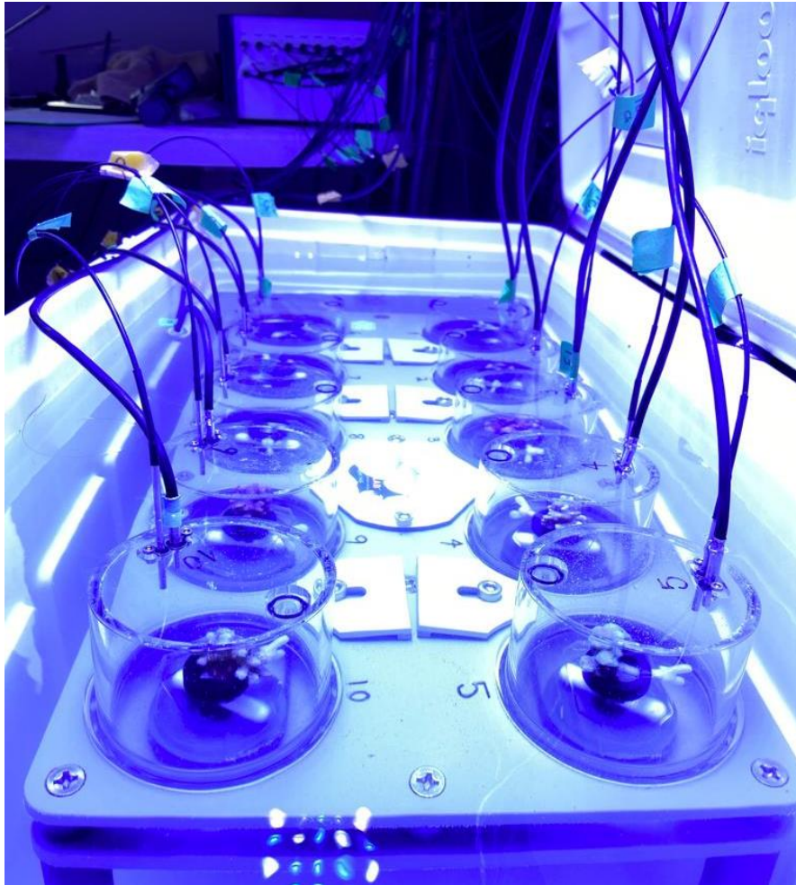
Figure 3. Respirometry setup: acrylic chambers are shown containing the coral fragments and spinners, connected to the Presens probes, and placed inside the cooler.
