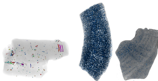
Figure 3.1: Reconstructed pieces with visible porosity
