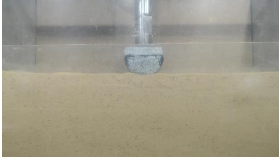
Figure 3. Test in the centrifuge with the rubber wheel.
