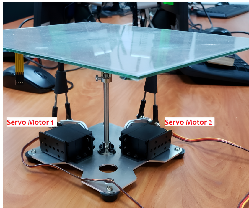
Figure 3.4: Servomotor identification in the Ball and Plate System.
