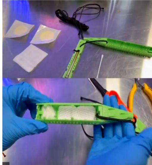
**Figure 5** Passive sampling 3D printed device (Schang et al., 2021)
