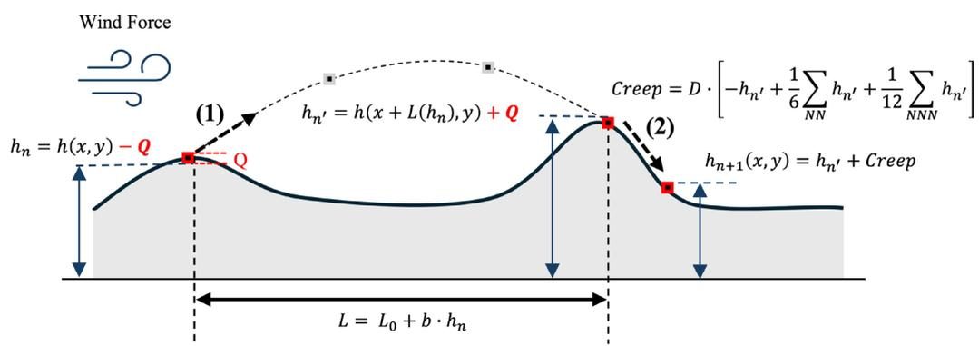
Figure 2 – Theoretical Model of Formation of Ripple Patterns by wind-blown sand
