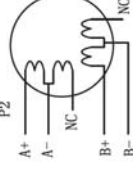
Figure 6: 6-lead motor half coil (higher speed) connections
