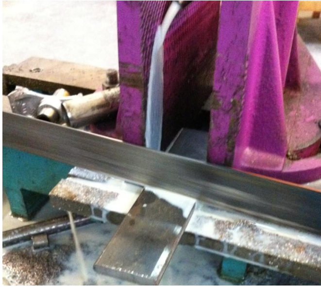
Figura 44: Sierra recortando material
