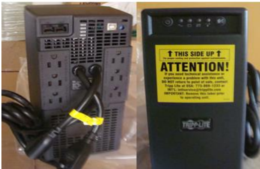
Figura 15 UPS (Uninterruptible Power Supply).
