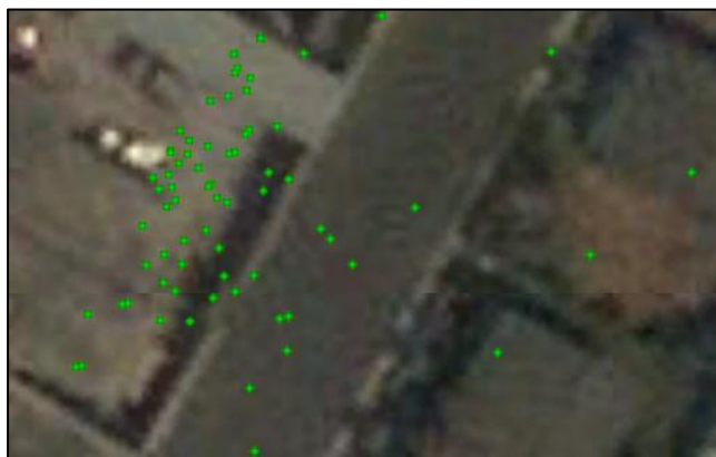
Figure 21.- Example of GPS data for a stationary vehicle
