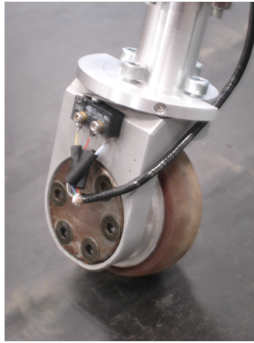
Figure 2.2: Binary contact switches
